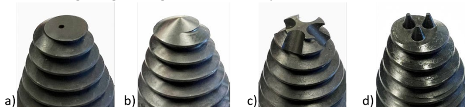
Fig. 2. Various FSEAM tool designs: a) flat bottom (current design with small hole for thermocouple), b) conical top, c) grooved, d) with pins. Designs b) – d) may be in contact with the build surface to enhance mixing and bonding.
