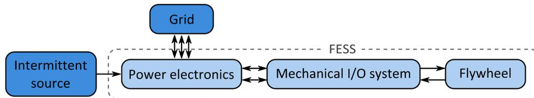
Figure 1: A typical scenario of a flywheel energy storage system connected to a local grid. I/O implies Input and Output.
