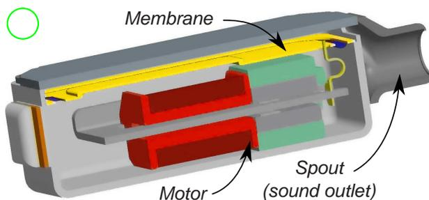
Figure 1 : Cross section of a hearing aid loudspeaker
