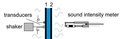
Figure 3 : Intensity measurements on double walls
