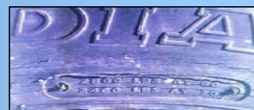
Fig. 1: Degradation (cracks) because of ozone attack on rubber
