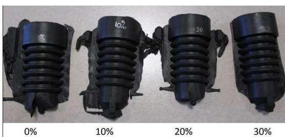
Fig. 1 : FKM sealing plugs with different percentages of devulcanized FKM.
