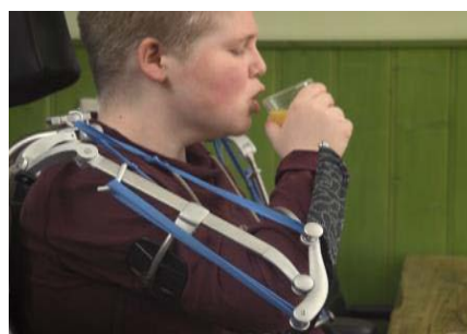
Fig. 1 : A Duchenne boy using an arm-lifting device with elastomer springs i.e. the blue strip.
