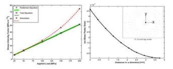
Figure 3 : Stress intensity calculation (left), von Mises plastic strain profile in x- direction (right)
