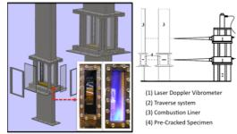
Figure 2 : Vibration-based monitoring on combustor.
