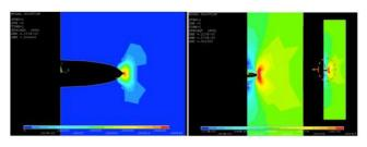
Figure 4 : Von Mises plastic strain field (left), von Mises elastic strain field (right) at the crack tip.
