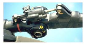
Figure 1 : External view of a lag damper
