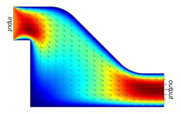
Figure 2 : Particle velocity in a 2D spout (real value)
