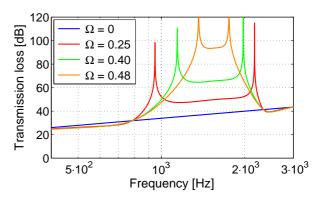
Figure 4 : Normal incidence sound transmission loss for different porosities
