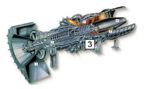
Figure 1 : Gas Turbine, 3 is the combustion chamber.
