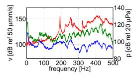
Figure 4 : Signal level for structural velocity (red), pressure in the combustion chamber (green) and pressure in the cooling passage (blue), see figure 2.
