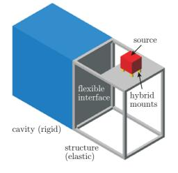
Figure 1 : Model of a hybrid isolation system.
