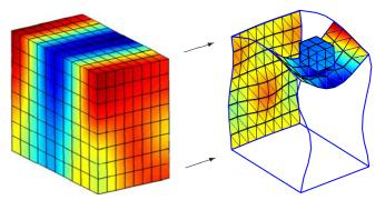
Figure 2 : Harmonic response of the cavity (excitated by the interface) and structure at 200 Hz.
