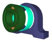
Figure 1 : Viscoelastic layer mounted between the bearing and the housing
