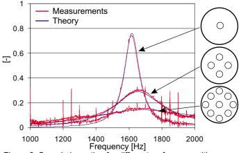
Figure 3. Sound absorption for different surface porosities.
