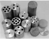
Figure 2. Sound absorbing samples.
