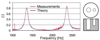
Figure 4. Sound absorption for two different perforations.
