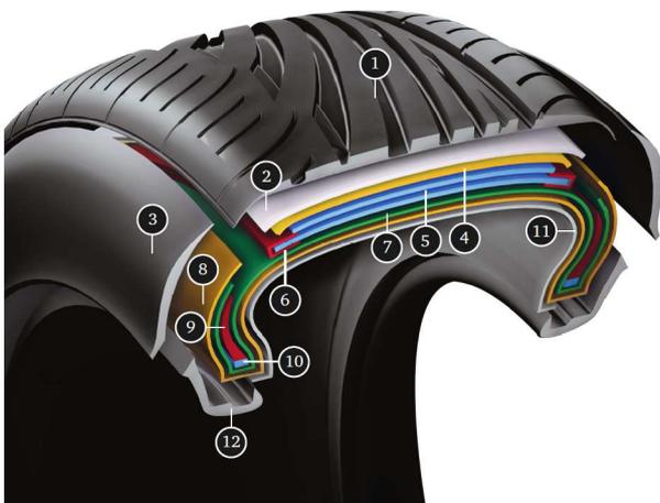
**Figure 1:** Cross-section of a radial tyre: tread (1), subtread (2), sidewall (3), NOH nylon overhead (4), belt layers 1 and 2 (5), belt rim tape (6), carcass layer 2 (7), carcass layer 1 (8), bead filler strip (9), bead (10), inner liner (11) and rubber rim band (12) (courtesy of Apollo Vredestein B.V.).
