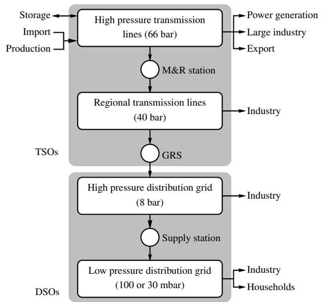
Fig. 1. Dutch gas grid supply chain
