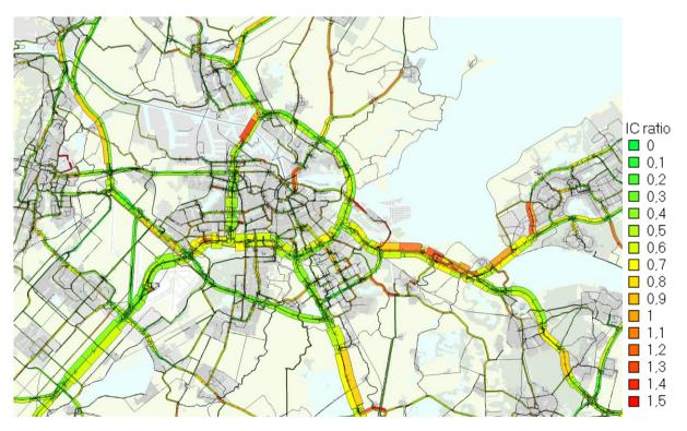
Figure 3.9: Network flows in the reference situation (width indicates flow, colour indicates I/C ratio)
