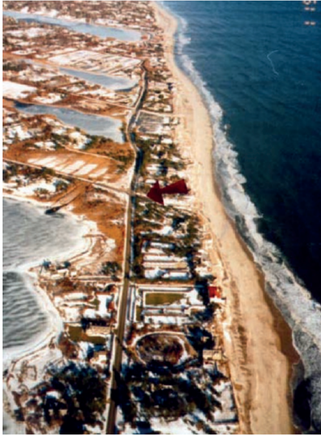
Figure 6.1: Alongshore shoreline sand waves at Southampton Beach, Long Island, NY. Extracted from Larson et al. (2002)
