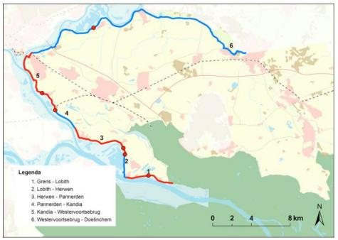
Figure 4 Dike sections where the final inundation extent is almost independent of the exact dike breach location in the section (Arends & Bisschop, 2014).
