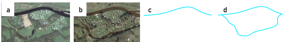
Figure 3.6. Side channel near Koeksebelt (a) before implementation (satellite), (b) after implementation (satellite), (c) before implementation (branches in model), and (d) after implementation (branches in model)
