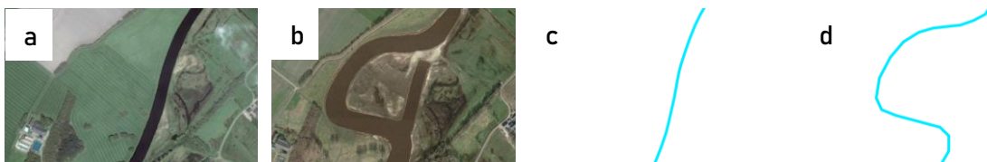
Figure 3.5. Meander near Karshoek-Stegeren (a) before implementation (satellite), (b) after implementation (satellite), (c) before implementation (branches in model), and (d) after implementation (branches in model)
