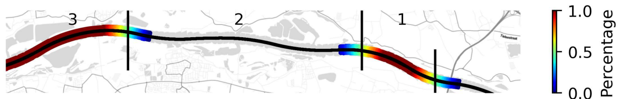
Figure 17 Transition zones between roughness sections to ensure smooth hydrodynamic effects. The roughness is interpolated between two adjacent roughness sections over a length of 2 km. The higher the percentage, the higher the contribution of the roughness section on a part of the river. Transition zones are shown for sections 1 and 3.
