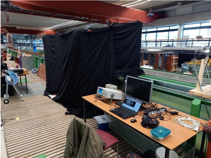
Figure 2-4, dark room tent placed over the wave flume for blocking light from the PIV measurement area.
