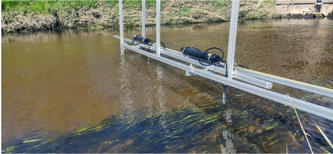
Figure 13 Overview of the experimental setup with the movable frame with two ADVs mounted. The length of the frame is 6 meters.
