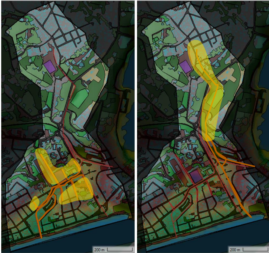
Figure 55 - Drainage systems (orange/red) in the catchment and upstream locations of drains in each system
