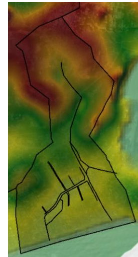
Figure 21 - DTM with drainage systems incorporated
