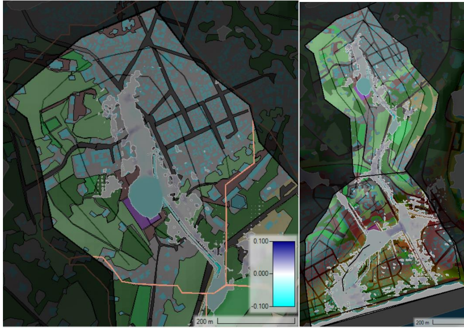
Figure 85 – Inundation maps of sub catchment 1 and the whole catchment for implementation of check dams
