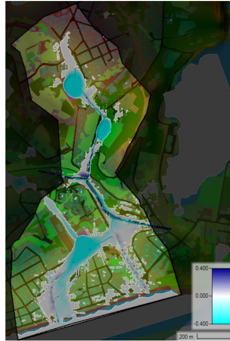
Figure 77 - Difference inundation map in comparison to the original situation when the northern part is separated
