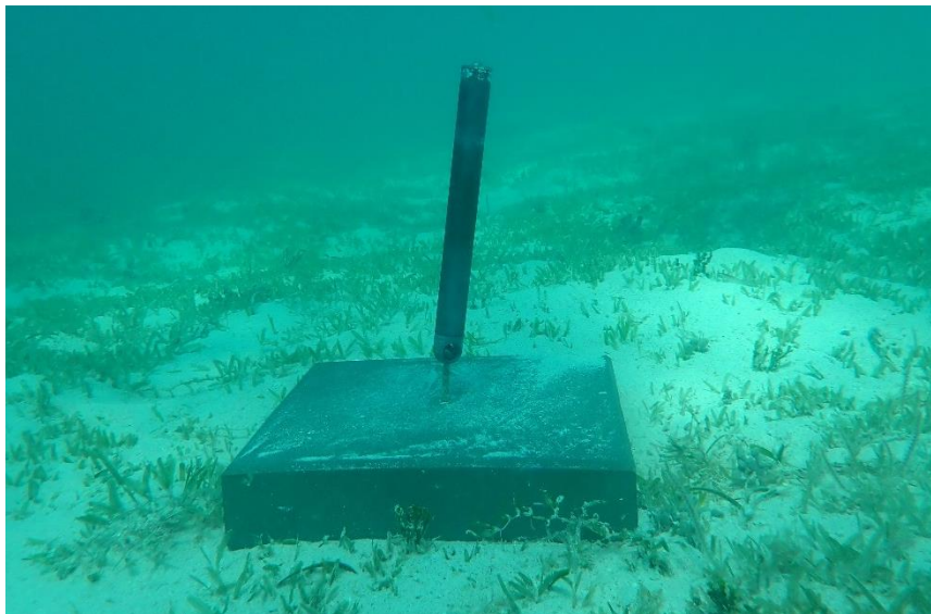
Figure 11: A Tilt Current Meter (TCM) attached to a paver near Cai
