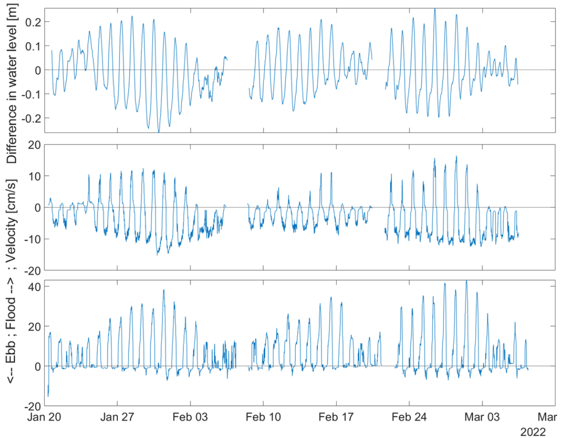
Figure 30: Water level difference between the forest fringe (WF) and Awa di Lodo (BW) (upper figure), the flow velocities in Kreek di Taco (EC) (middle figure) and the flow velocities in Kreek di Pedro (WC) (lower figure)
