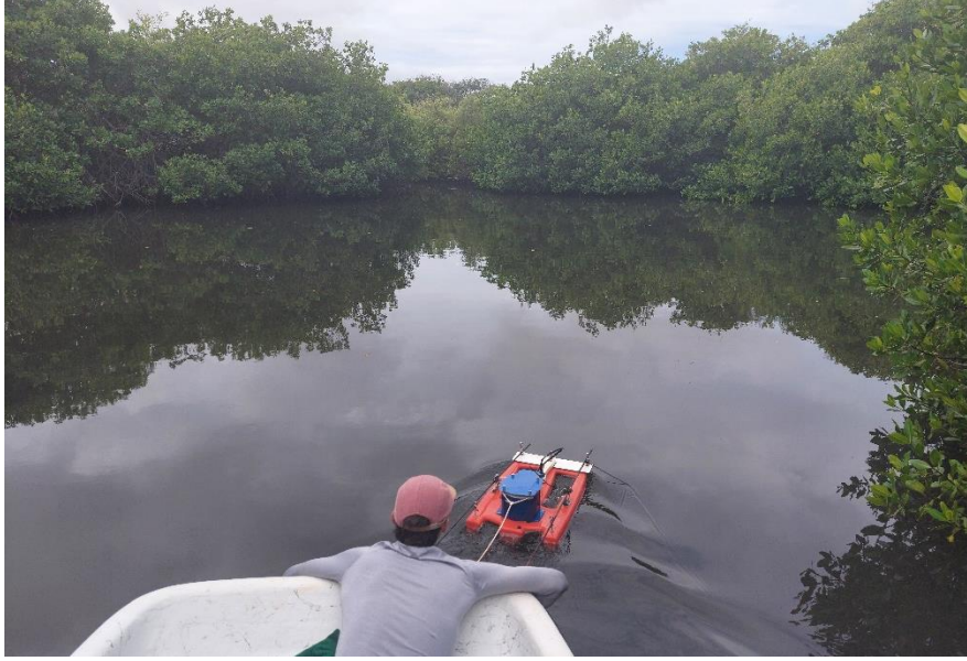
Figure 10: Gathering water depth data with the ADCP in the creeks of Lac Bay
