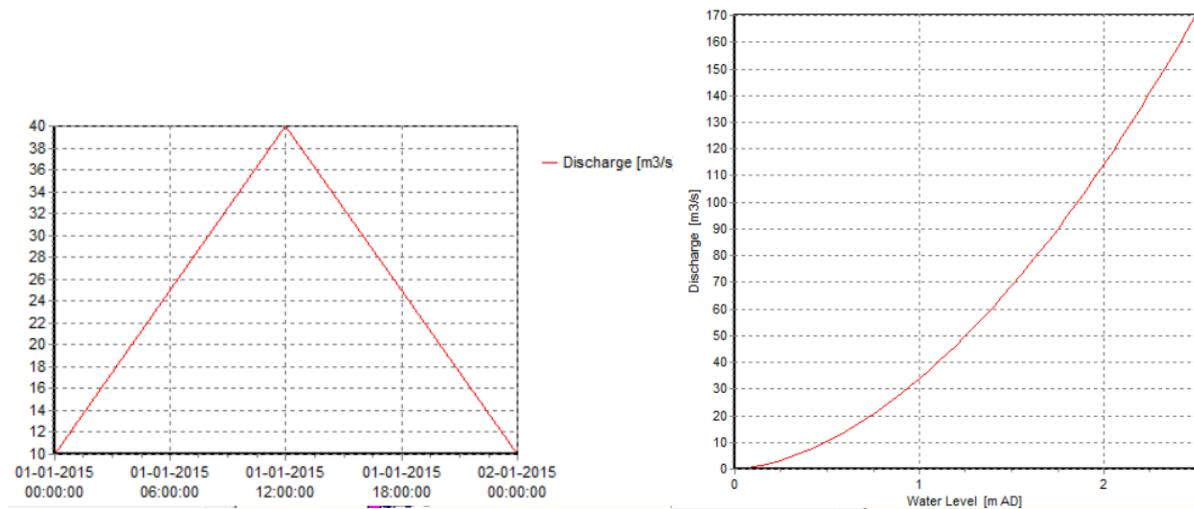
Figure C-2 - left: incoming flood wave; right: Q-h relation
