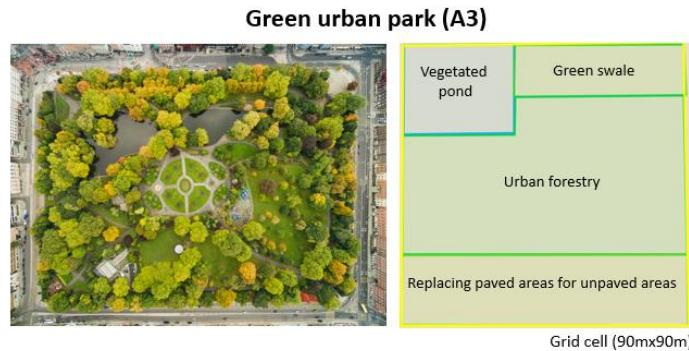
Figure C- 5 - schematisation of a green urban park in a grid cell in AST
