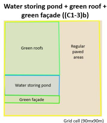
Figure C- 6 - schematisation of a water storing pond, green roofs and green facade in a grid cell in AST
