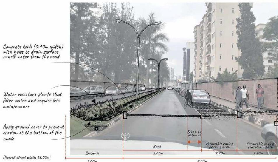
Figure C- 8 - integrated road profile / green blue spine (B1 & C5) (World Bank, 2021)
