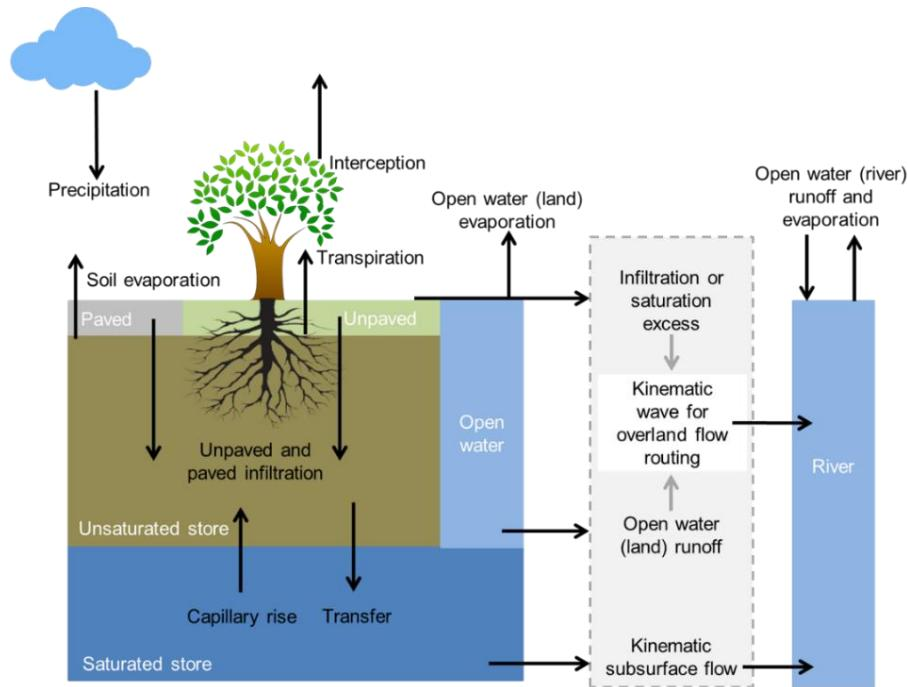
Figure 5 - overview of the wflow-SBM concept (Schellekens, 2019)
