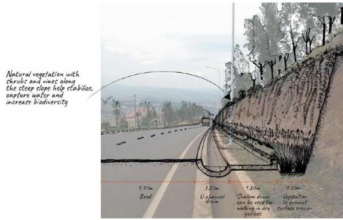
Figure C- 10 - green integrated drain (D5) (World Bank, 2021)
