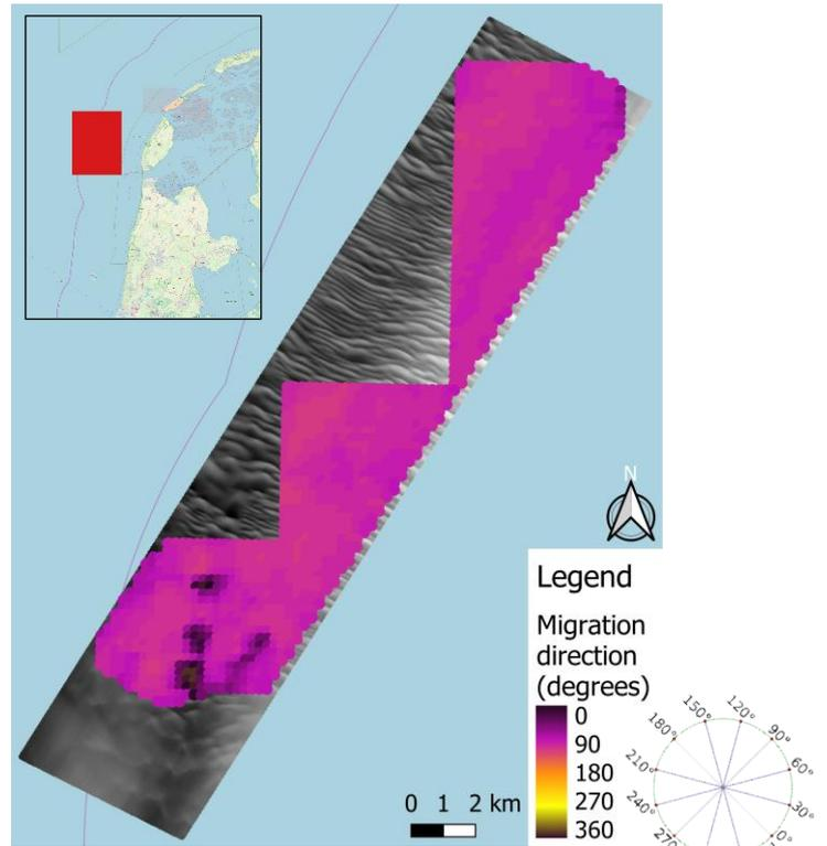
Figure 52 Spatial distribution of migration directions by SCC (weighted regression vector, window size 36) for West of Texel
