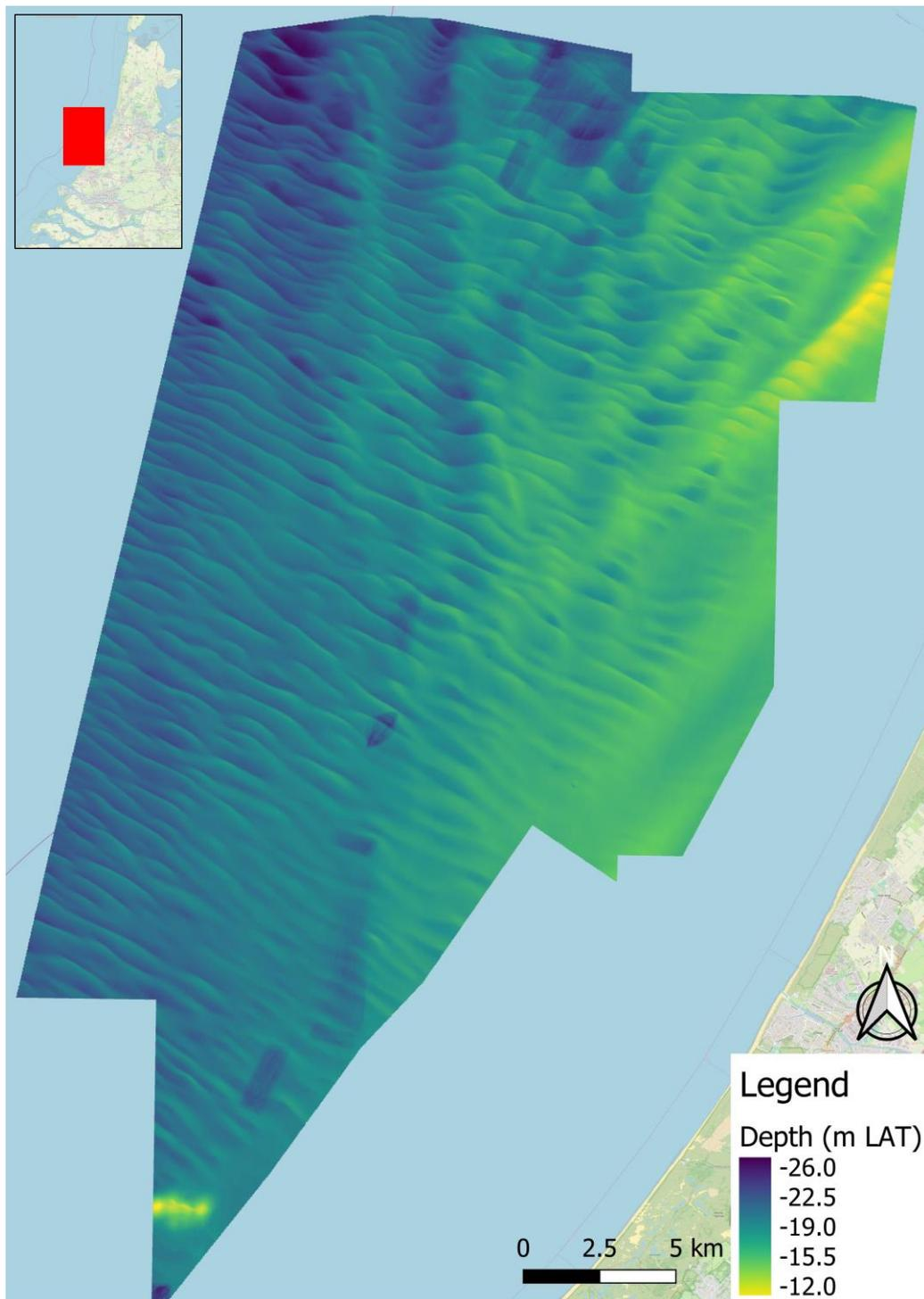
Figure 48 Bathymetry at field site IJmuiden-Hoek van Holland
