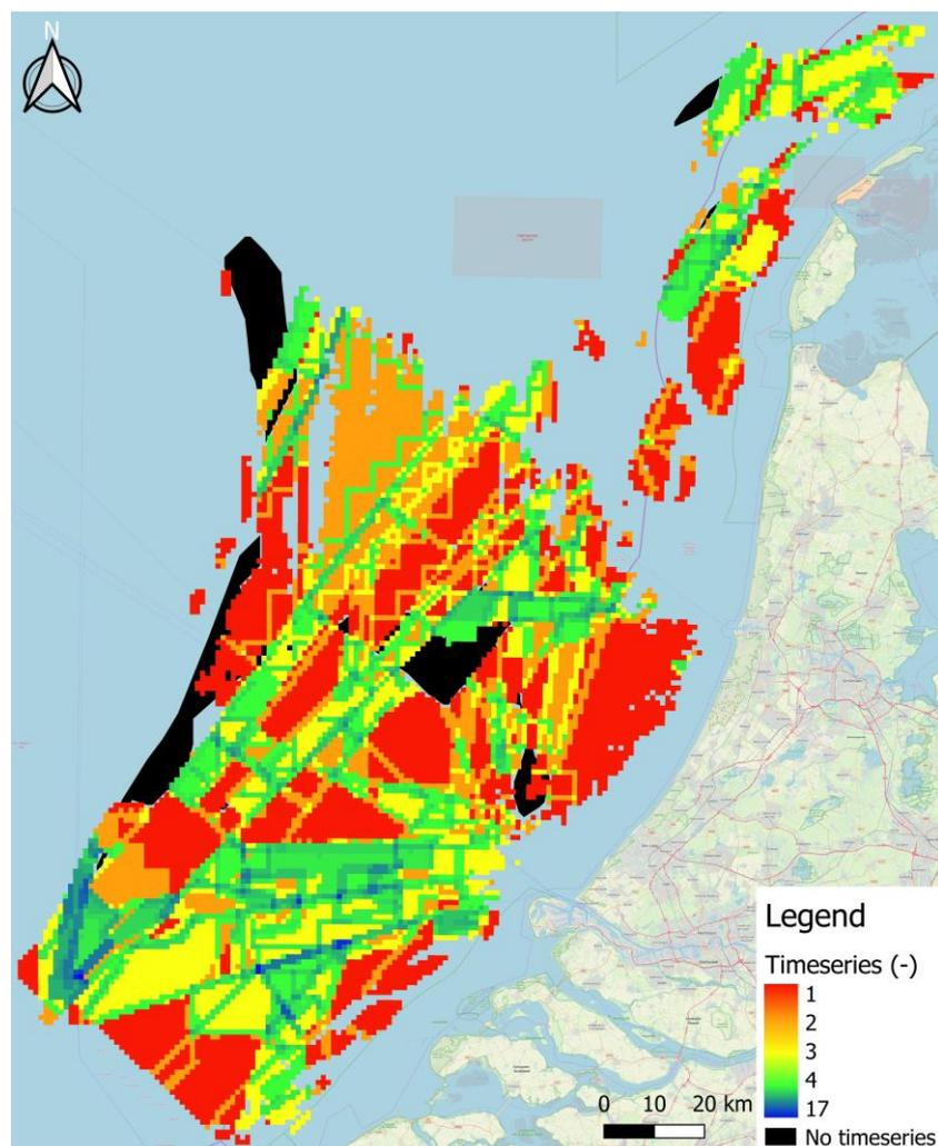
Figure 73 Number of timeseries per km<sup>2</sup> (1 timeseries = 2 bathymetric datasets)
