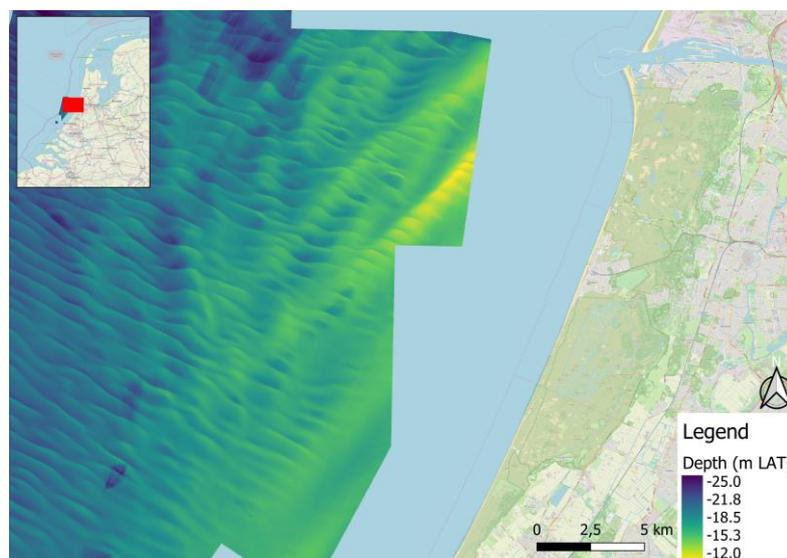
Figure 1 Bathymetry near the coast of IJmuiden
