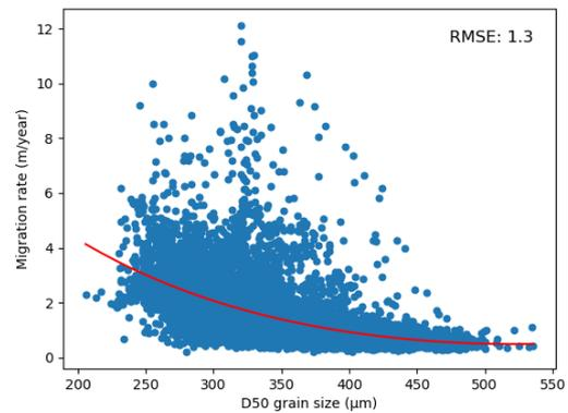
Figure 83 Migration rate per km<sup>2</sup> (m/year) plotted against D50 grain size per km<sup>2</sup> (µm)
