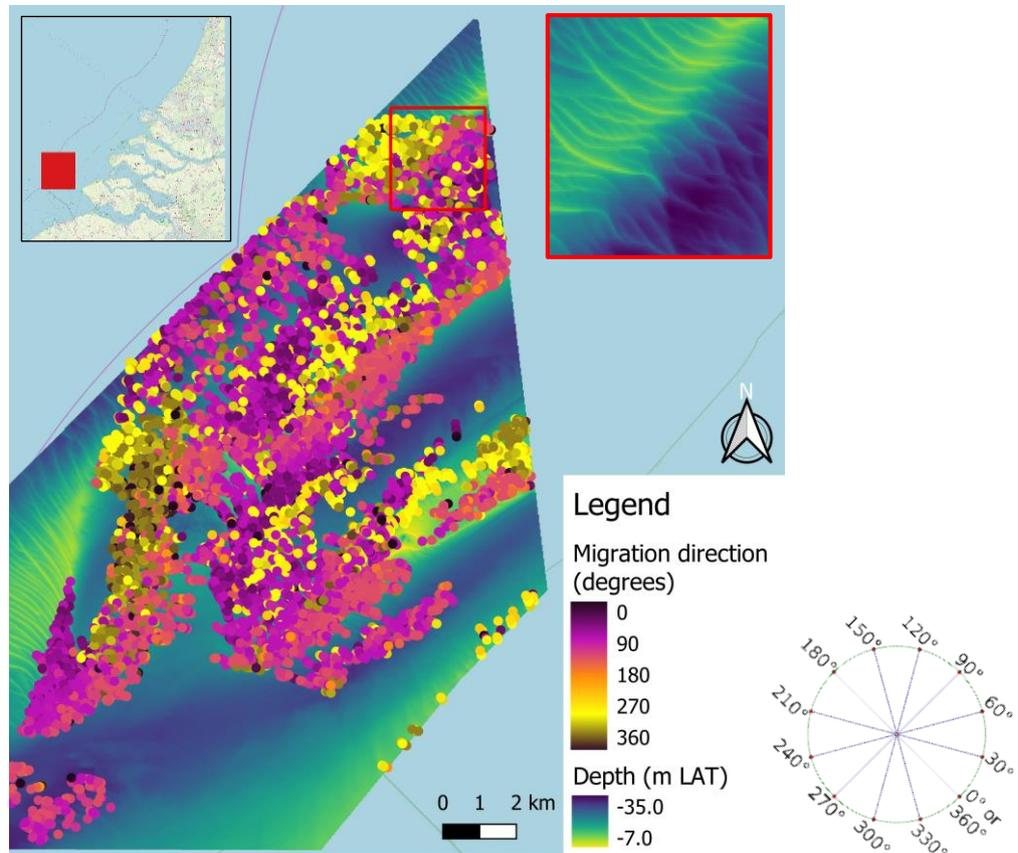
Figure 80 Migration directions, bathymetry, and sand wave orientation (red square) at Schaar-Rabsbank
