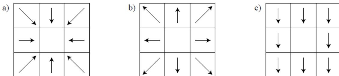
Figure 34 The convergence index is calculated based on aspect. The averages of the relative aspects are (a)  $0^\circ$ , (b)  $180^\circ$  and (c)  $90^\circ$ . The convergence indexes are  $-90^\circ$  (a),  $90^\circ$  (b) and  $0^\circ$  (c) (Kiss, 2004).
