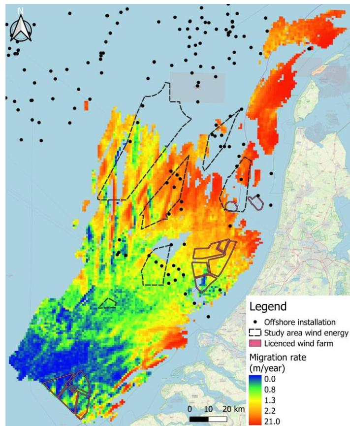
Figure 90 Average sand wave migration rate per km<sup>2</sup>, present and future windfarms and offshore installations
