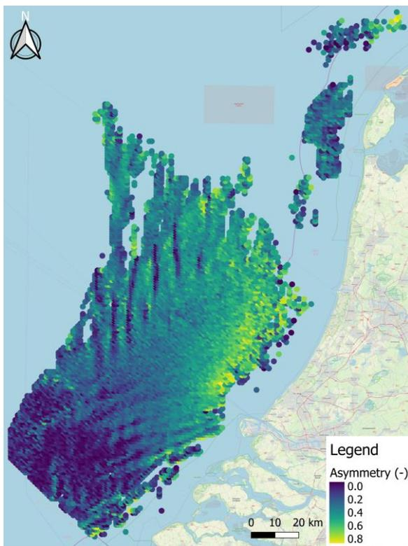
Figure 15 Sand wave asymmetry per km<sup>2</sup>
