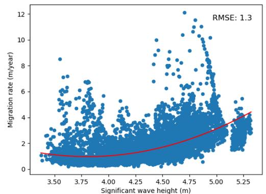
Figure 85 Migration rate per km<sup>2</sup> (m/year) plotted against significant wave height per km<sup>2</sup> (m)
