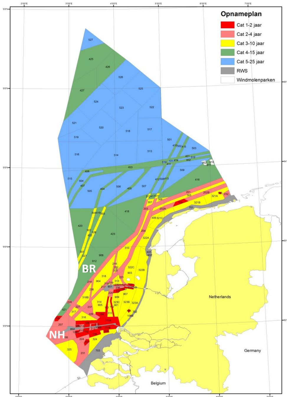
Figure 86 Re-survey strategy of the Netherlands Hydrographic Office. North Hinder and the Brown Ridge are abbreviated with NH and BR, respectively (Netherlands Hydrographic Office, 2021b).
