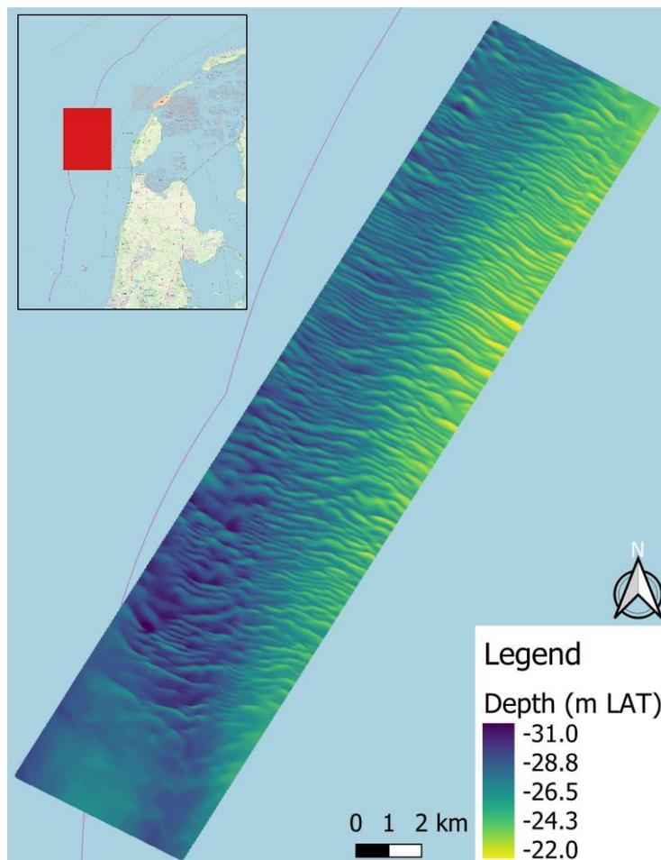
Figure 45 Bathymetry at field site West of Texel
