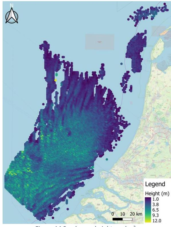
Figure 14 Sand wave height per km<sup>2</sup>
