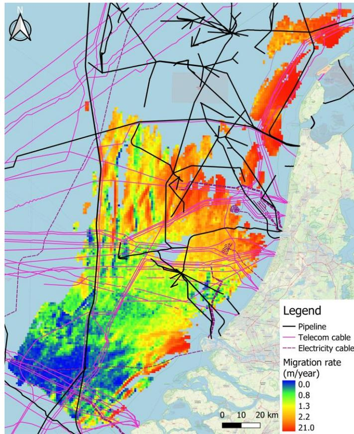
Figure 89 Average sand wave migration rate per km<sup>2</sup>, pipelines and cables
