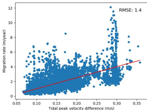
Figure 84 Migration rate per km<sup>2</sup> (m/year) plotted against tidal peak velocity difference per km<sup>2</sup> (m/s)
