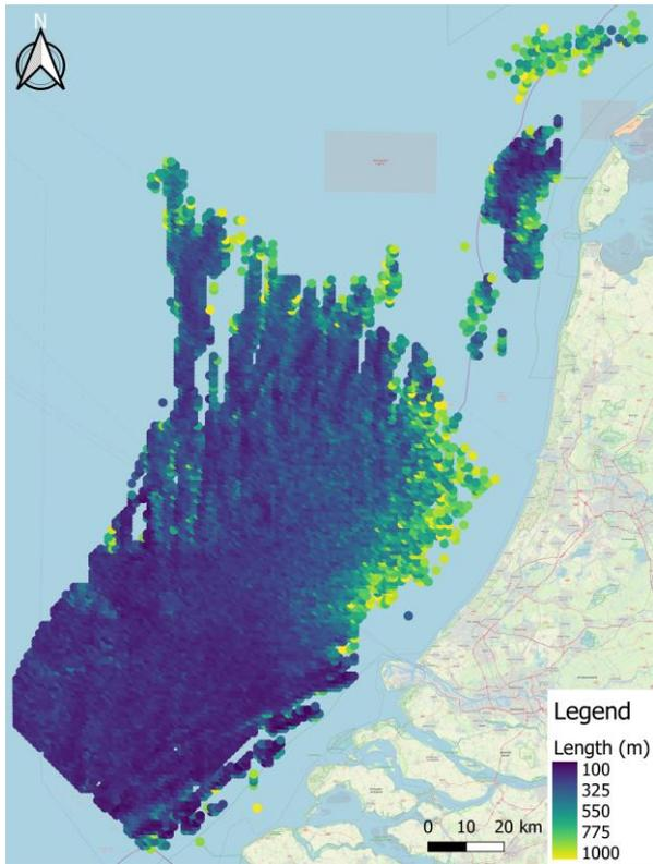
Figure 13 Sand wave length per km<sup>2</sup>
