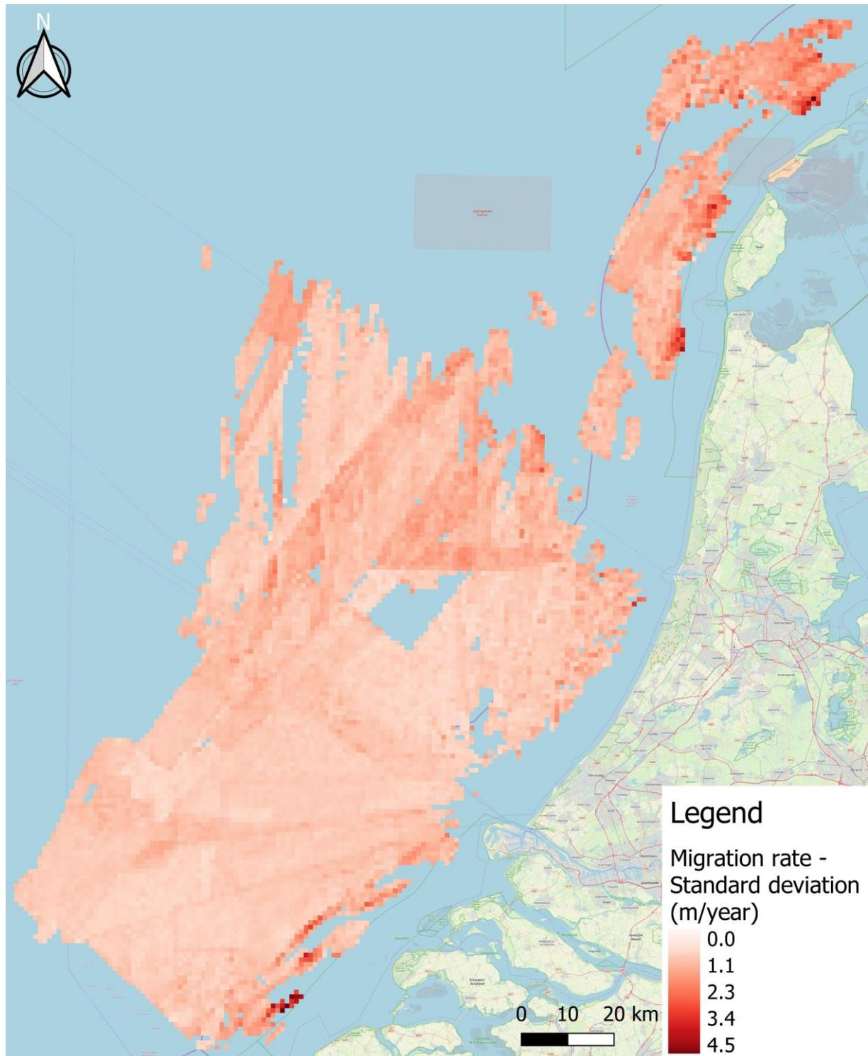
Figure A7.1 Standard deviation of migration rate per km<sup>2</sup>
