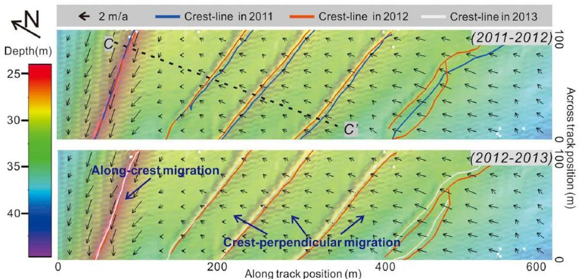
Figure 20 Migration vectors as obtained with the cross-correlation technique (Zhou et al., 2018)
