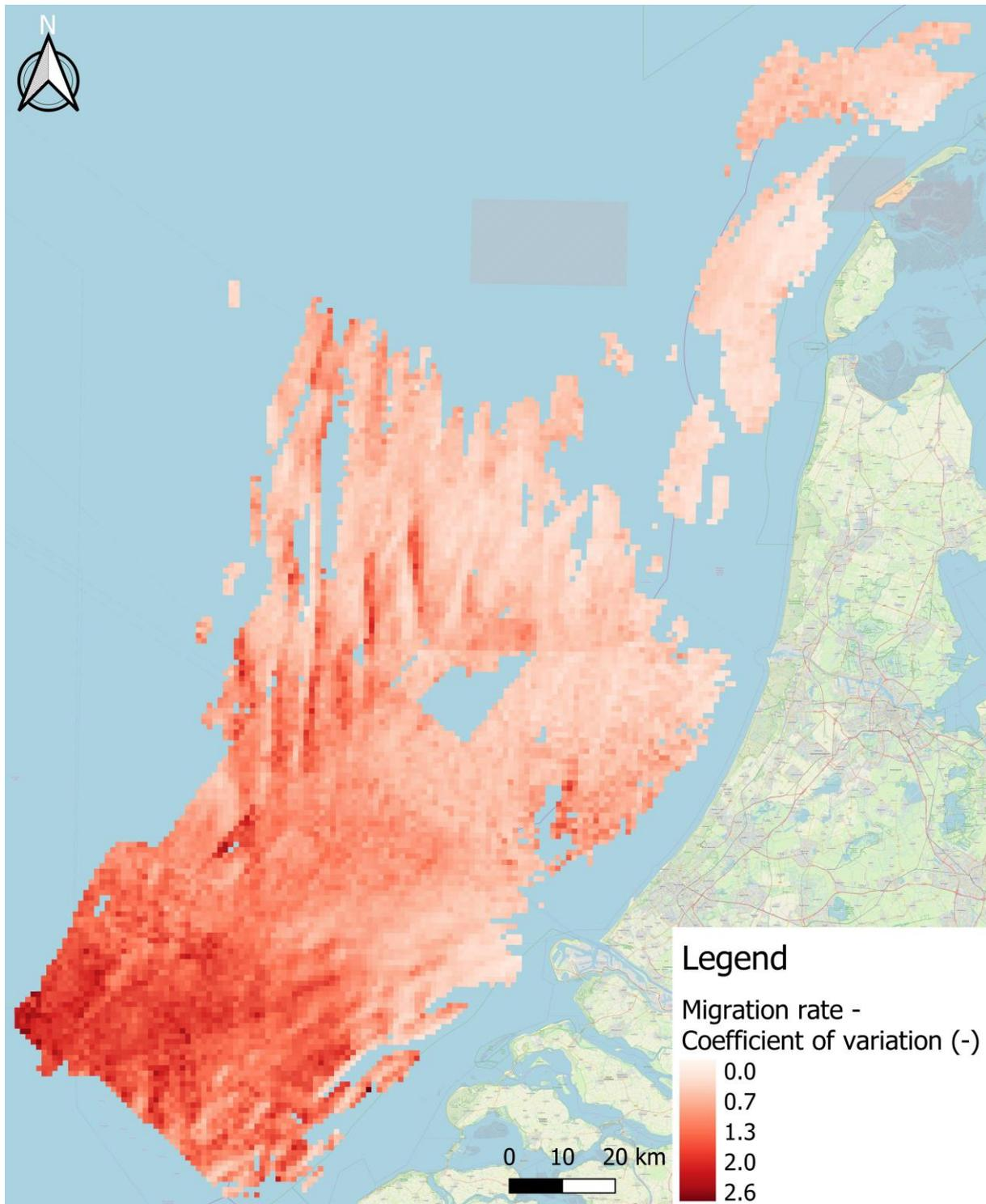
Figure 79 Coefficient of variation (standard deviation/mean) of migration rate per km<sup>2</sup>
