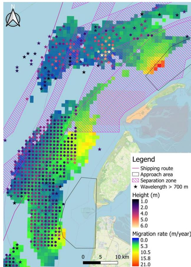
Figure 88 Average sand wave migration rate and height per km<sup>2</sup> at the Wadden Islands, including shipping routes (Rijkswaterstaat, 2021).
