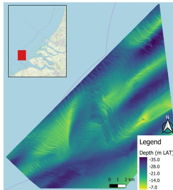
Figure 46 Bathymetry at field site Schaar-Rabsbank
