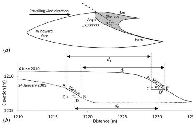
Figure 26 Quantifying dune migration based on slip face displacement ( $d_0$ ) (Dong, 2015)
