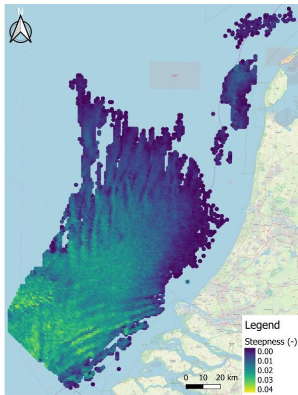
Figure 16 Sand wave steepness per km<sup>2</sup>
