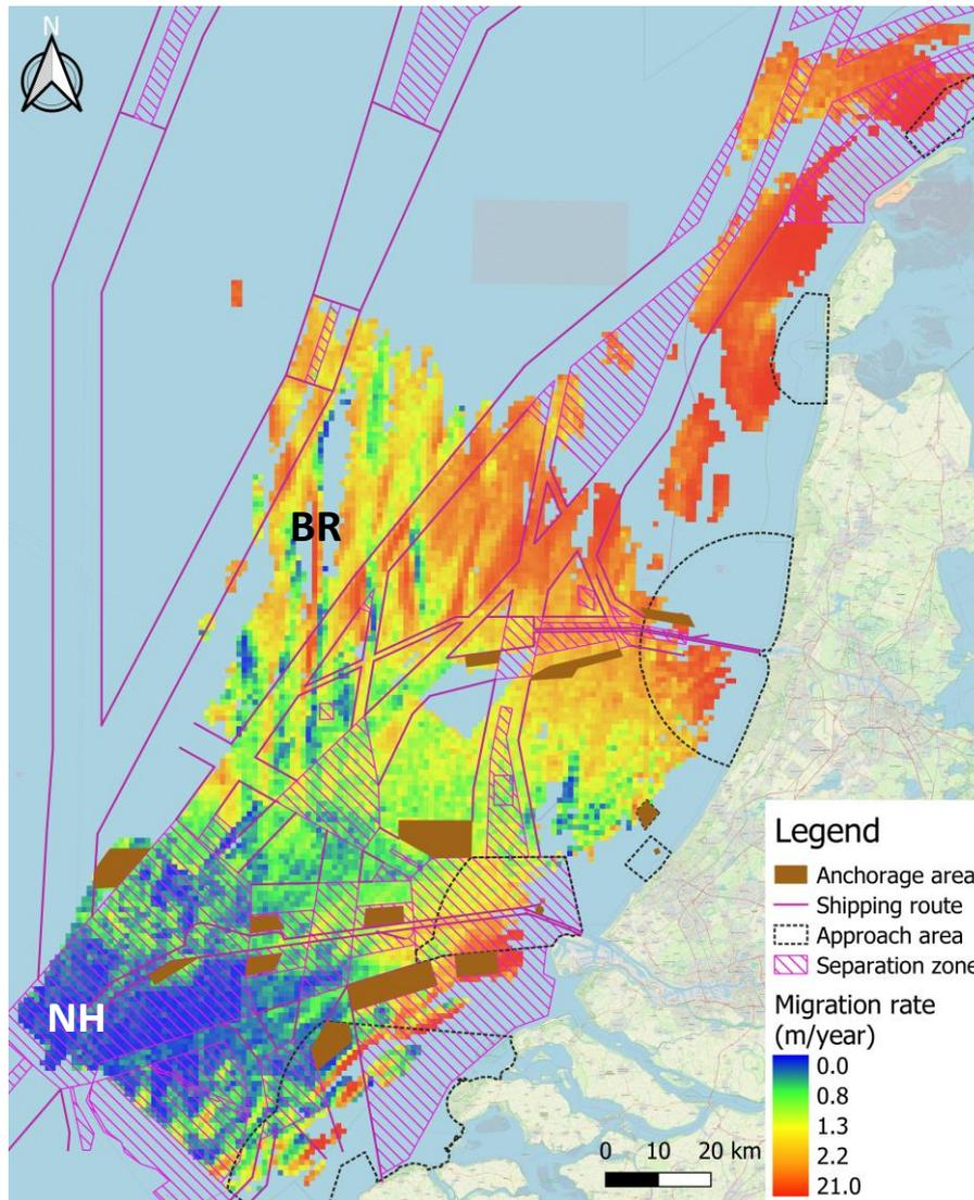
Figure 87 Average sand wave migration rate per km<sup>2</sup> and shipping routes on the NCS. North Hinder and the Brown Ridge are abbreviated with NH and BR, respectively (Rijkswaterstaat, 2021).
