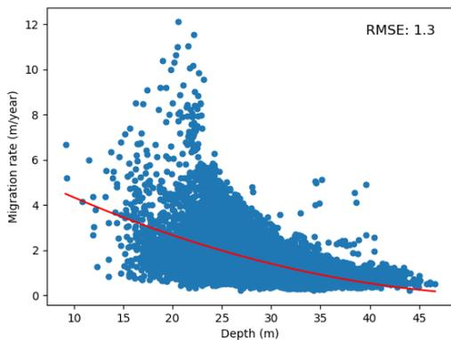
Figure 82 Migration rate per km<sup>2</sup> (m/year) plotted against depth per km<sup>2</sup> (m)
