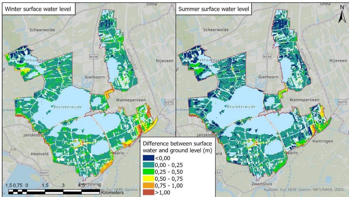
Figure 12: Summer and winter drainage level (difference between surface water level and ground level) in meter.
