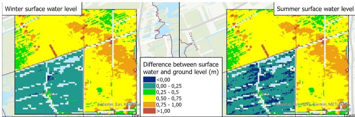
Figure 14: Close up of the focus area showing the difference in winter and summer drainage level in meter.
