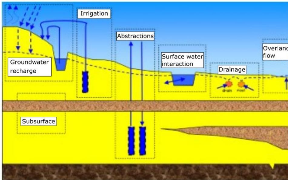
Figure 5: Modelled processes in the MIPWA/MODFLOW groundwater model
