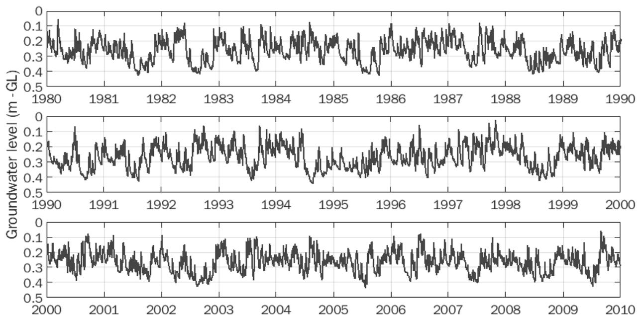
Figure 10: Spatially averaged groundwater level (m – GL) for the reference situation (1981-2010) excluding all surface water.
