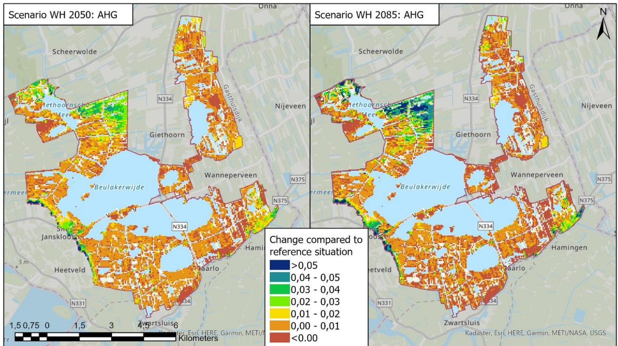
Figure 20: Predicted change in AHG (m) for scenario WH in 2050 and 2085 compared to the reference situation. A negative value means that the AHG decreases (further away from ground level).
