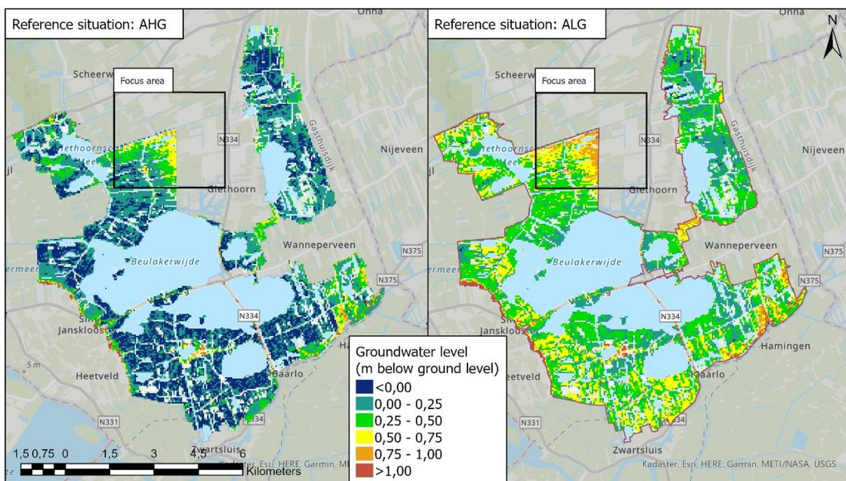
Figure 11: AHG and ALG for the reference situation (m – GL). The focus area represents an area with different GWL and is clarified below.
