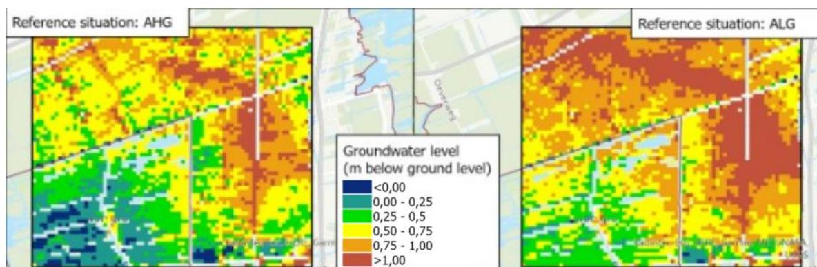
Figure 13: Close up of the focus area showing the AHG and ALG for the reference situation (m - GL).
