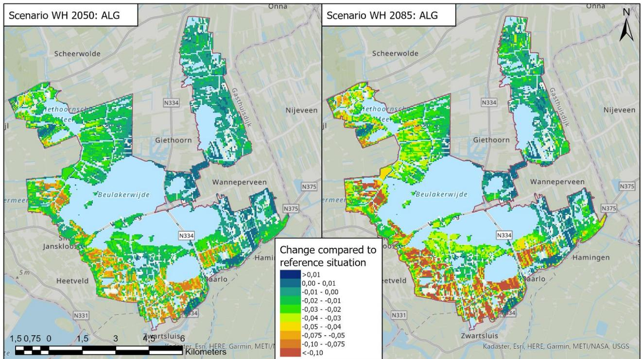
Figure 21: Predicted change in ALG (m) for scenario WH in 2050 and 2085 compared to the reference situation. A positive value means that the ALG increases (closer to ground level).
