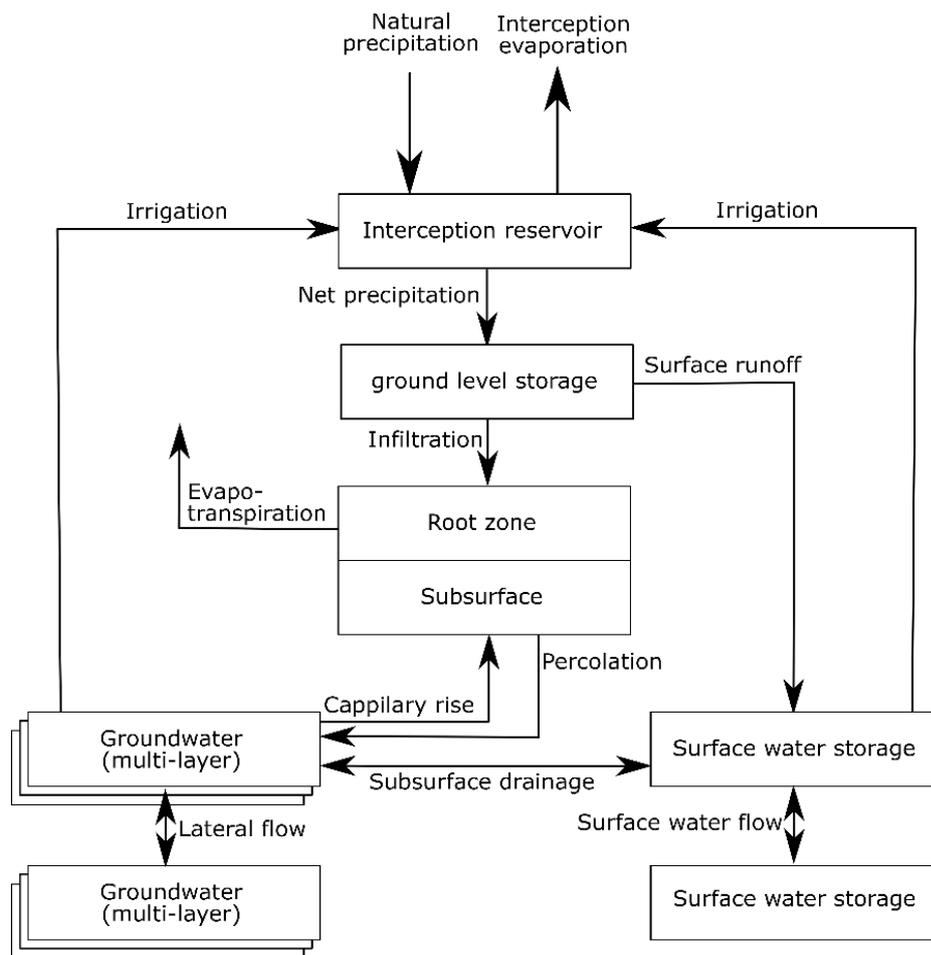
Figure 6: Conceptual model for simulating groundwater recharge using the CAPSIM module (Snepvangers et al., 2007).
