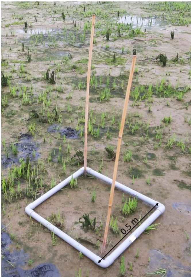
Figure 3: Measurement set-up of the vegetation plots (0.5 x 0.5 m) on the Marconi salt marsh. The erosion pins mark the two diagonal corners of the vegetation plot for consistency of the measurements over the growing season. Every field trip, the erosion pins were measured, five Salicornia plants in the vicinity of each vegetation plot were analysed, and a photo was taken from above the vegetation plot to determine the FVC.
