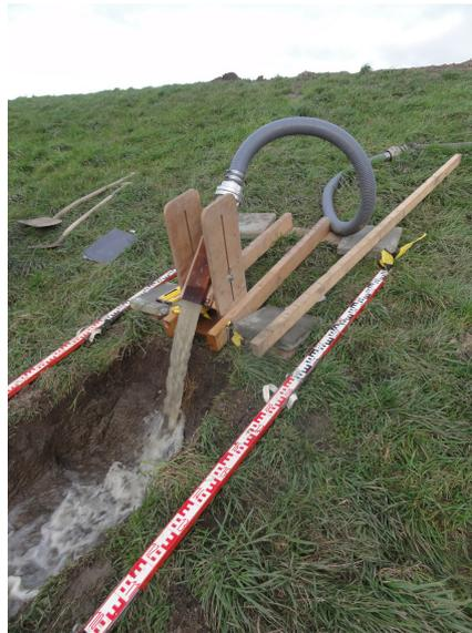
Figure 1.3: Setup of the fire hose method experiment.
