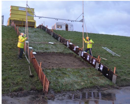
Figure 3.6: Wave overtopping experiment performed in the Hedwige-Prosperpolder.
