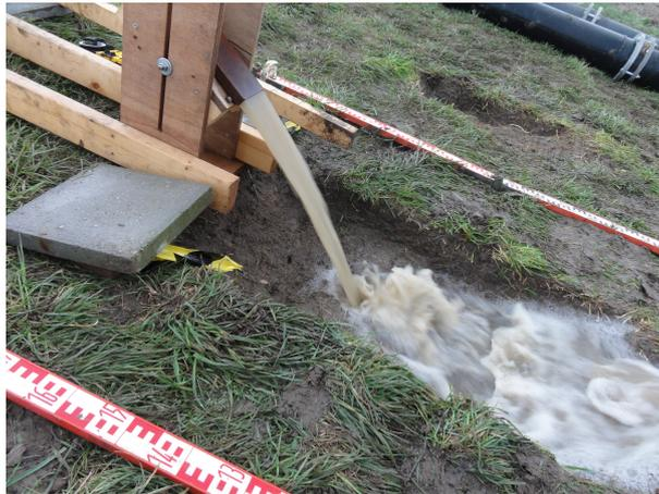
Figure 5.5: Spreading of the flow after the jet impacts.
