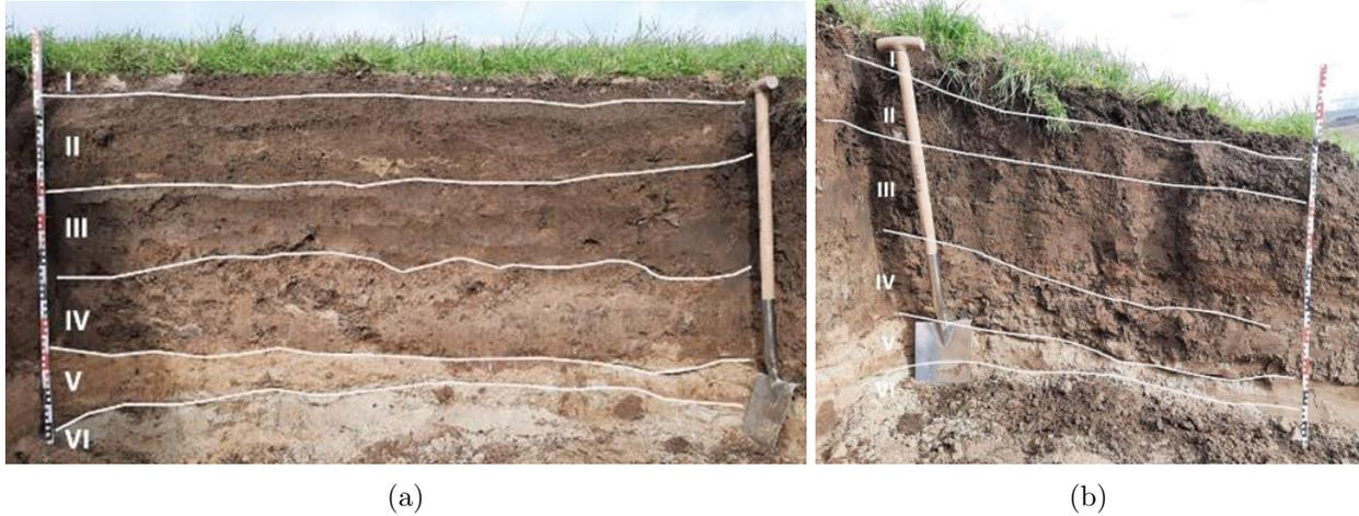
Figure D.2: (a) Back wall and (b) side wall of ‘Proefkuil West’ (Koelewijn, 2022). The division between each layer is indicated with a white line.
