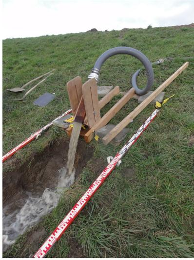
Figure 3.2: Fire hose method experiment performed in the Hedwige-Prosperpolder.
