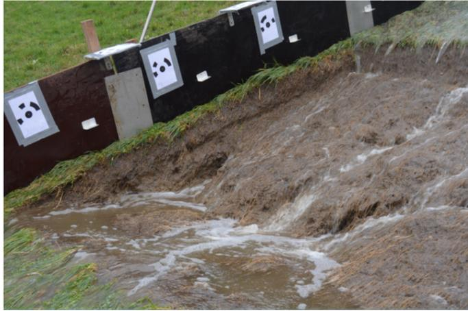
Figure 4.8: Picture of the erosion at the bottom of hole after the wave overtopping experiments were finished.
