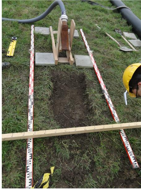
Figure 5.4: Measuring raster used during fire hose method experiments.
