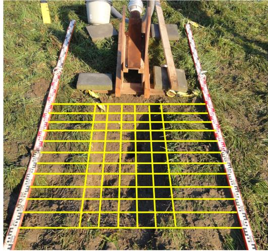
Figure B.4: Measuring points at erosion hole every ten centimeters.
