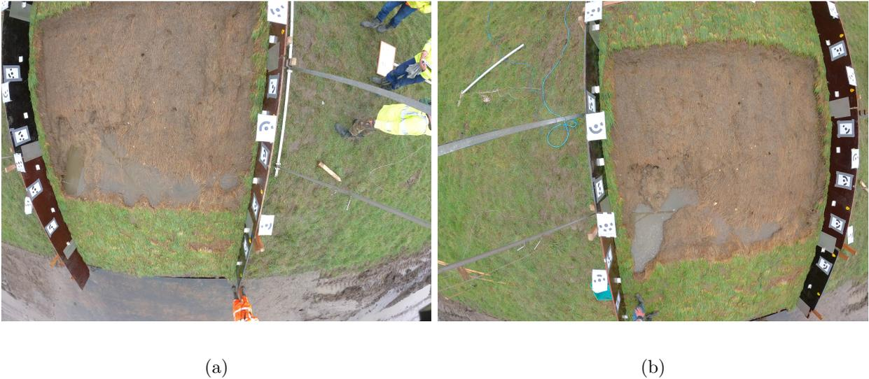
Figure 5.7: Images used for photogrammetry (a) before and (b) after 10 waves of 2000 L/m were released.
