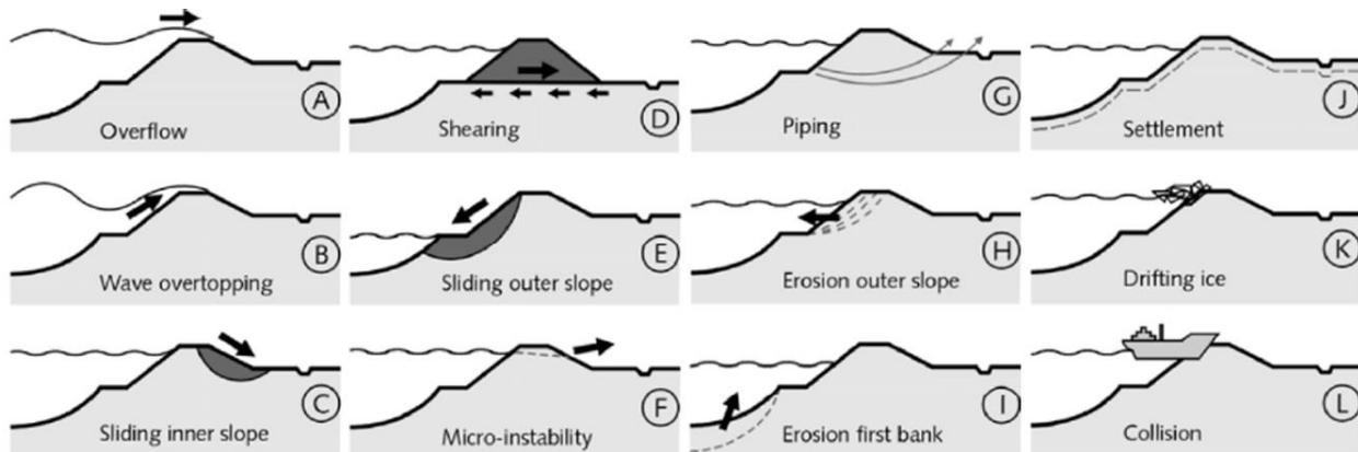
Figure 3. Failure mechanisms of soil structures (TAW, 1998)
