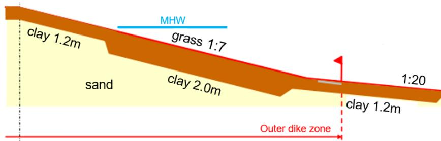
**Figure 12.** Wide green die design (adapted from van Loon-Steensma & Schelfhout (2013))
