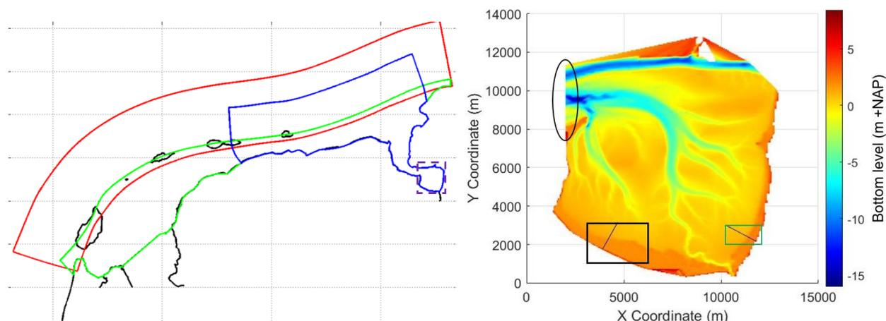
**Figure 14.** Map of different grids of the background SWAN model of the Wadden Sea as used for the input of Hydra-NL (left map). Bathymetry Dollard basin with study area and segment of WGD in the black rectangle, boundary segment in the oval and study area and segment of location in Germany in the green rectangle (right map).
