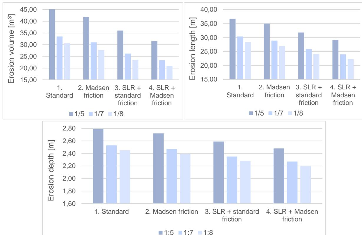
Figure 33. Results erosion hole and clay layer thickness for the different scenarios and dike slope
