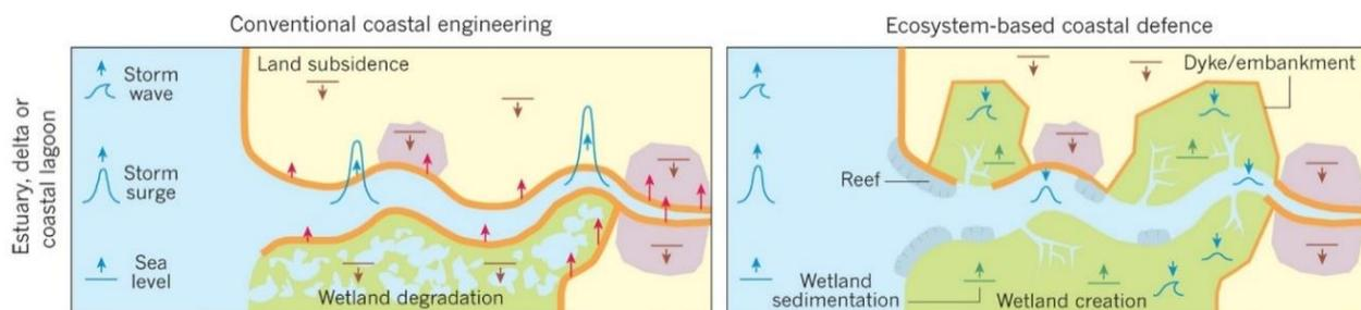
**Figure 8.** Conventional versus nature-based coastal defence (Temmerman et al., 2013)
