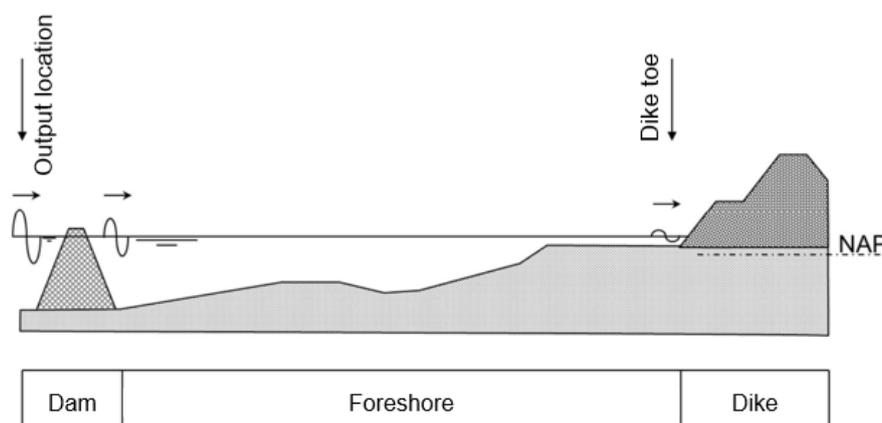
**Figure 36.** Schematisation Dam and Foreshore module Hydra-NL (Rijkswaterstaat, 2019)
