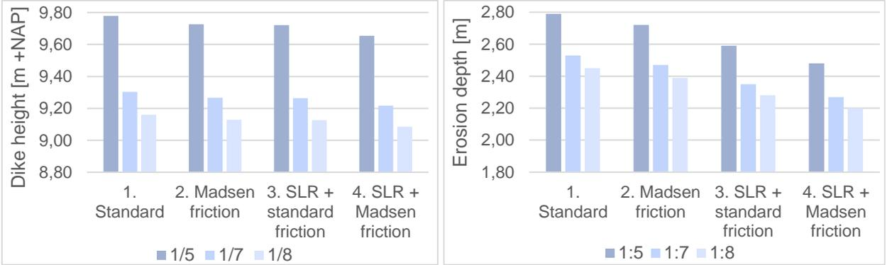
Figure 2. Required dike dimensions for different scenarios
