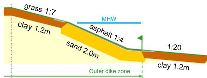
Figure 11. Current (traditional) dike design (adapted from van Loon-Steensma & Schelfhout (2013))
