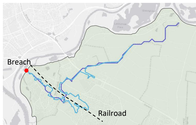
Figure 39 – Flow paths on 10x10m resolution (light blue) and 150x150m resolution (dark blue) in first time step
