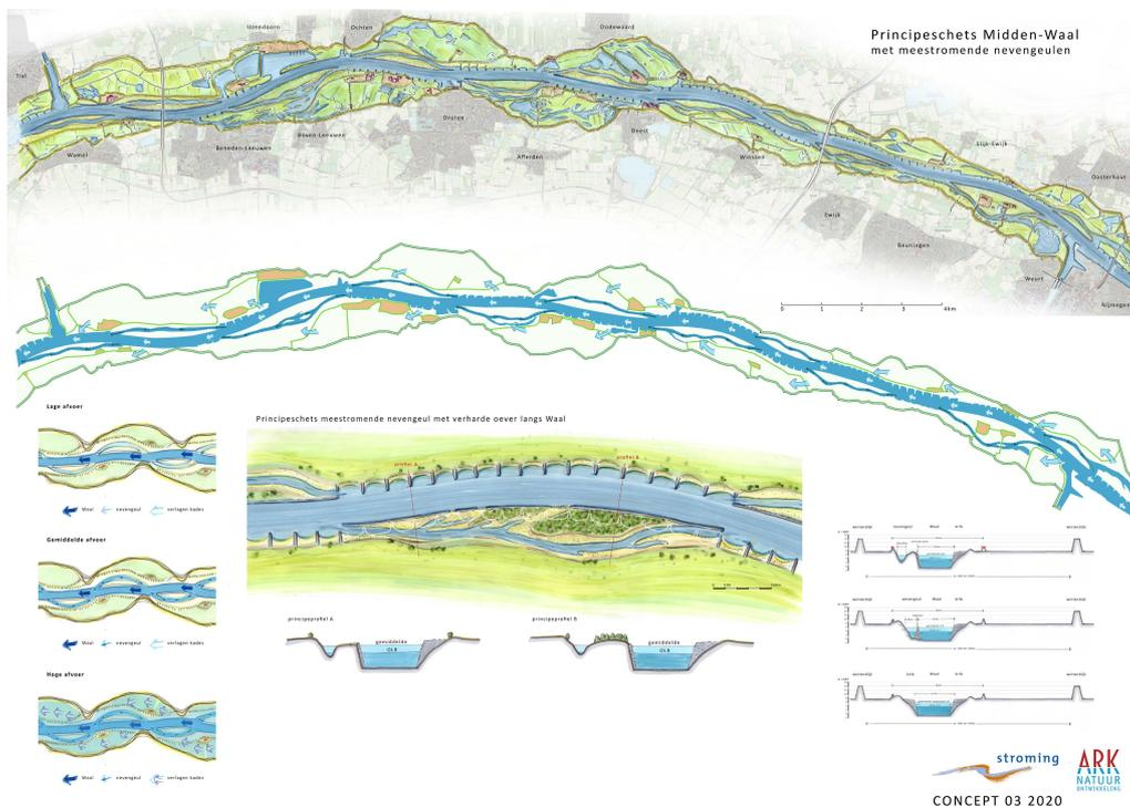
Figure 1: Conceptual drawings of the river within the Room for Living Rivers vision (ARK Natuurontwikkeling and Bureau Strooming, 2020). Top: an artist impression of the RfLR vision. The three drawings bottom left: the flow profile for different types of discharge. Bottom center: a more detailed view of a side channel. Bottom right: cross sections of three different river sections.
