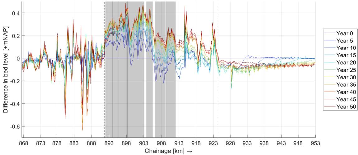
Figure 19: Width averaged bed level difference for every five years. The locations of the side channels are marked in grey, while the black dashed lines indicate the boundary of the floodplain lowering.
