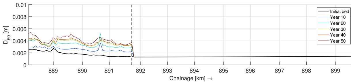
Figure 10: Development of the width averaged  $D_{50}$  in the reference scenario in time. The dashed line indicates the domain boundary where the bed sediment composition and sediment transport equation changes.
