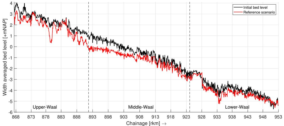
Figure 8: Bed level in the reference simulation initially and after fifty years. The dotted lines indicate the domain boundaries.
