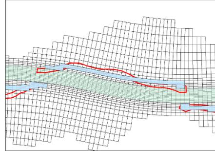
(c) Model grid with sketched side channel outline (red), schematized side channel (blue) and main channel (green).
