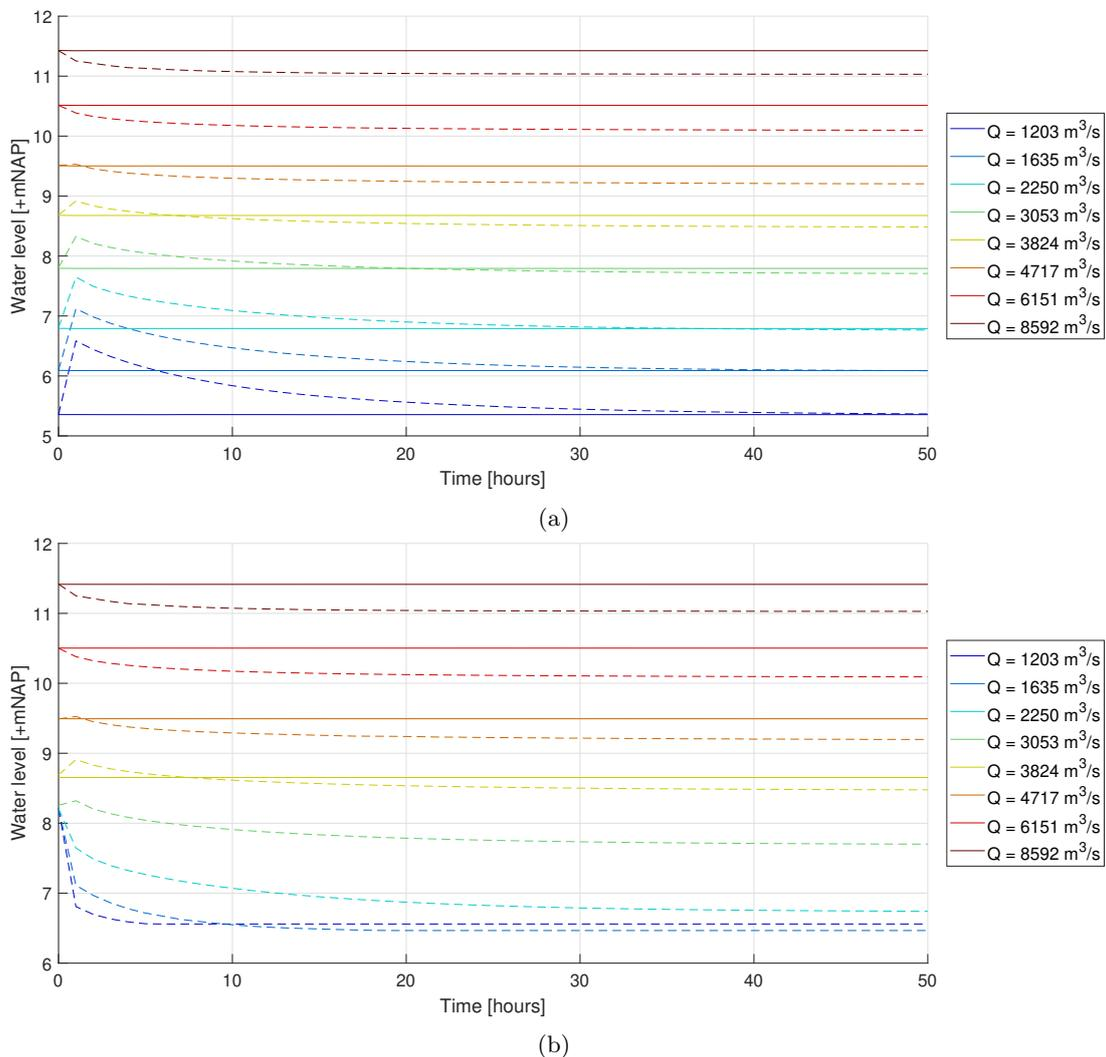
Figure 26: Simulated water levels over time without morphological development for all simulated discharges (a) at rkm 893 in the main channel and (b) in the newly incorporated side channel. The solid and dashed lines represent the reference scenario and the RfLR scenario respectively. No water levels are shown for discharges below  $3053 \text{ m}^3/\text{s}$  for the reference scenario in (b), as this location is a non-inundated floodplain in the reference scenario.
