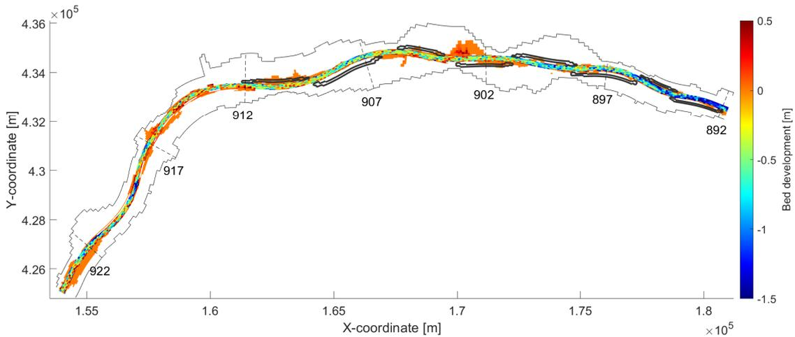
Figure 15: Bed level change in the Middle-Waal after fifty years including the RfLR measures. In black the location of the side channels are shown. The dashed lines indicate the riverkilometer.
