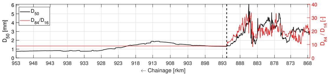
Figure 4: Width averaged characteristics of the initial bed composition in the River Waal:  $D_{50}$  (left axis) and the non-uniformity of the sediment given by  $D_{84}/D_{16}$  (right axis). The dashed line indicates the border between the domain using graded sediment (right side) and the uniform sediment (left side).
