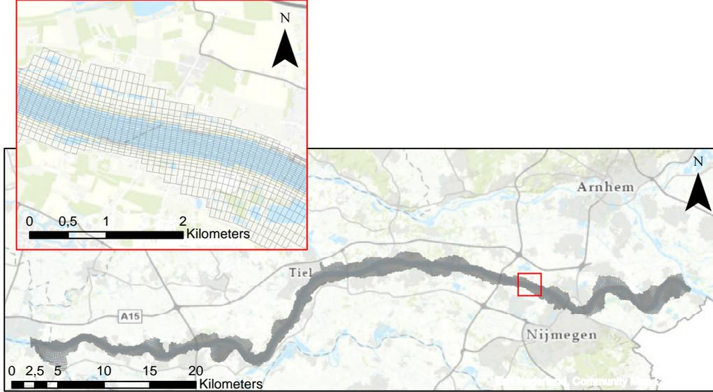
Figure 3: Numerical grid covering the river Waal. Background image adapted from Esri Nederland.
