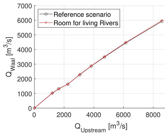
Figure 13: Discharge distribution at the bifurcation Pannerdensche Kop from which the River Waal originates for both the reference and Room for Living Rivers scenario.
