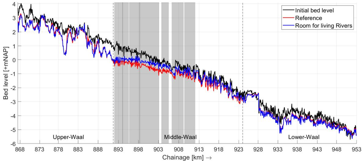
Figure 20: Width averaged bed level of the main channel initially and after fifty years for both scenarios. The locations of the side channels are marked in grey. The black dashed lines indicate the boundary of the floodplain lowering.
