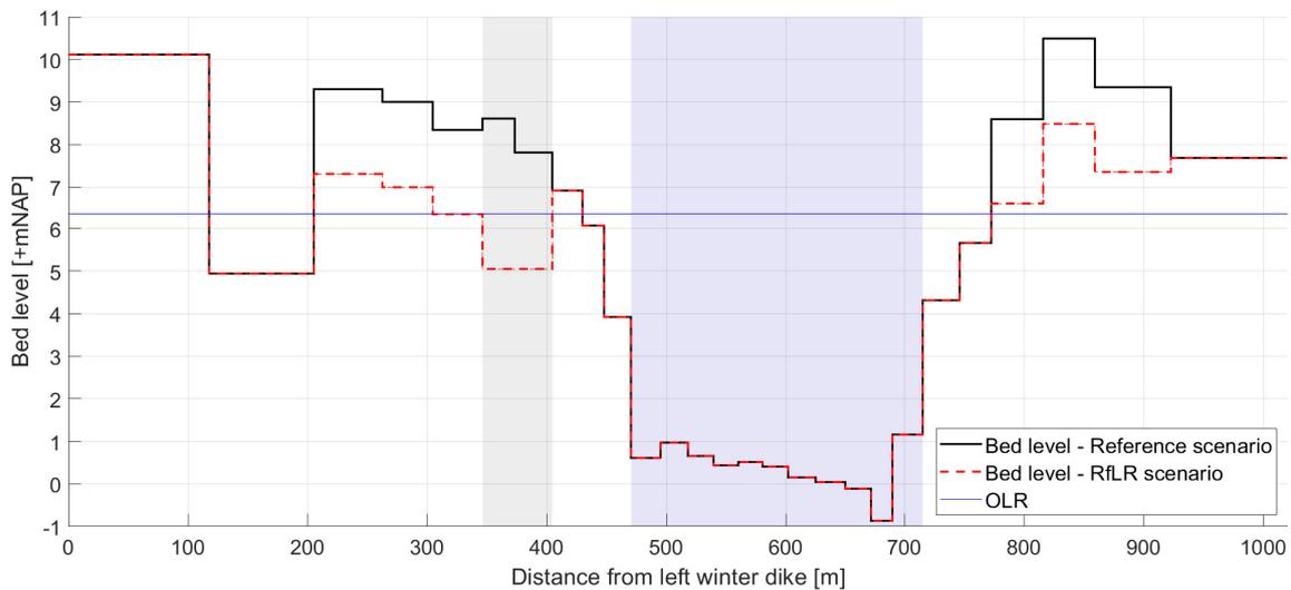
Figure 11: Cross-section of the river bed level at rkm 893 for both scenarios. The shaded areas indicate the two channels: main channel (blue) and the new side channel (grey). The floodplains within 100 m of the dike remain unaltered, while the rest of the floodplains have been lowered by 2 m, with OLR (blue line) as minimum floodplain level. The bed of the side channel lies 1.2 m below OLR and the area between the side and main channel is left as currently present.
