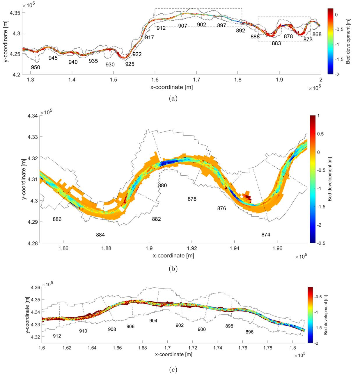
Figure 7: Bed level development of the river Waal in the reference scenario over fifty years. The dashed lines indicate the riverkilometers. The direction of flow is from right to left. (a) River waal from the Pannerdensche Kop until Gorinchem. The boxes indicate the areas zoomed in below. (b) Zoom of the river section between rkm 870 and 888 (right box). (c) Zoom of the river section between rkm 892 and 913 (left box).
