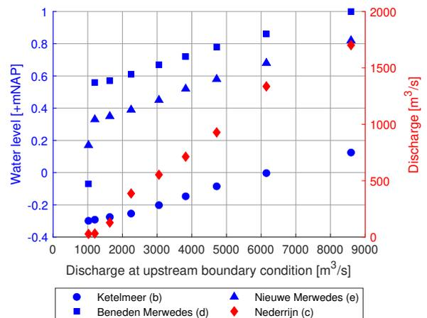
Figure 6: The applied downstream boundary conditions. The letter between parenthesis corresponds to the locations marked in Figure 2. Adapted from Yossef et al. (2008).
