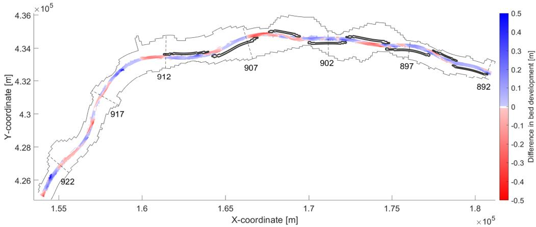
Figure 18: Difference in initial bed level response due to the river interventions between the Reference and RfLR scenario after one year. Negative values indicate more erosion in the RfLR scenario. Flow direction is from right to left.
