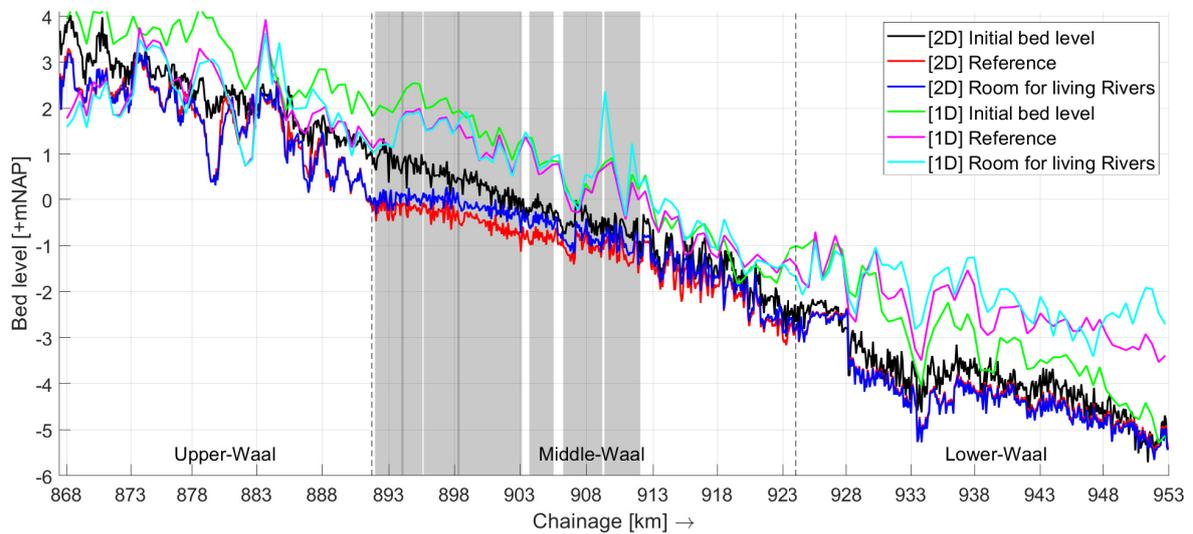
Figure 23: Initial bed level and bed level after 50 years for the two scenarios in the current 2D study compared to the modelled bed levels initially and after 100 years of an earlier 1D study by Barneveld et al. (2019).
