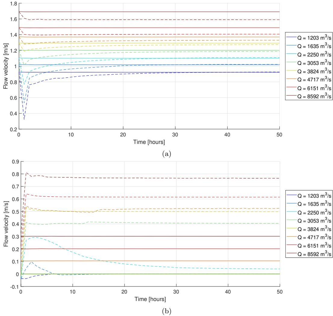
Figure 27: Simulated flow velocities over time without morphological development for all simulated discharges (a) at rkm 893 in the main channel and (b) in the newly incorporated side channel. The solid and dashed lines represent the reference scenario and the RFLR scenario respectively. No flow velocities are shown for discharges below 3053 m<sup>3</sup>/s for the reference scenario in (b), as this location is a non-inundated floodplain in the reference scenario.
