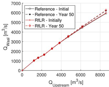
Figure 21: The discharge distribution at the Pannerdensche Kop initially and after fifty years for both the reference and the RfLR scenario.
