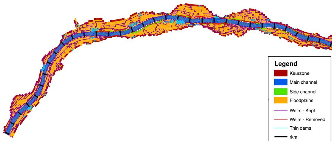
Figure 25: Room for Living River schematization regarding classification of cells and sub-grid structures.
