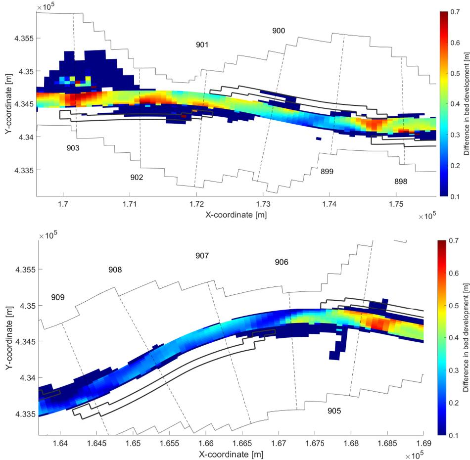
Figure 17: Close-up view of the difference in bed development after fifty years between both scenarios between rkm 897 and 903 (top) and between rkm 904 and 910 (bottom).
