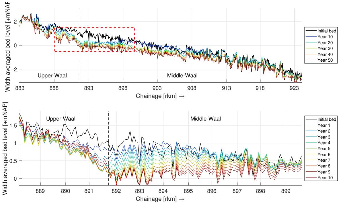
Figure 9: Bed level development in the reference scenario in time. The dashed line indicates the domain boundary where the bed sediment composition and sediment transport equation changes. Top: Every ten years, bottom: zoom to area marked by red rectangle.
