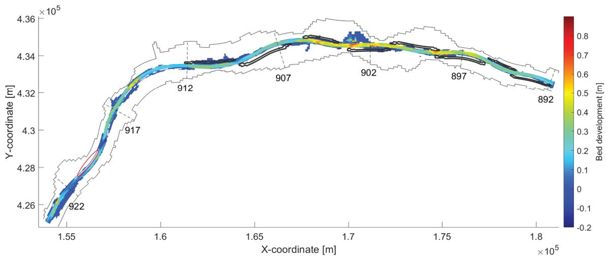
Figure 16: Difference in bed development after fifty years. The bed level in the reference scenario is subtracted from the RfLR scenario; hence a positive value implies less erosion in the RfLR scenario. The dashed lines indicate the riverkilometer, the red circle encircles the only area where the RfLR measures induce additional erosion compared to the reference scenario.
