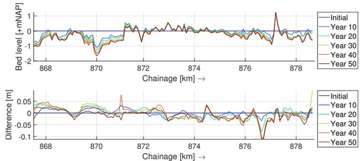
Figure 22: Top: width averaged bed level in the Pannerdensch Kanaal initially and after each ten years in the reference scenario. Bottom: difference in width averaged bed level in between reference and RfLR scenario. A positive value indicates less erosion in the RfLR scenario.
