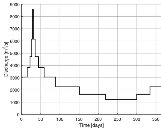
Figure 5: The annual discharge hydrograph as applied at the model upstream boundary. This hydrograph is repeated for fifty years. Adapted from Yossef et al. (2008).
