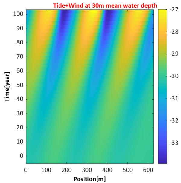
Figure 32: Sand wave evolution in the presence of tidal and severe wind conditions for 100 years at 30m mean depth. The vertical colour bar shows the bed level (m).
