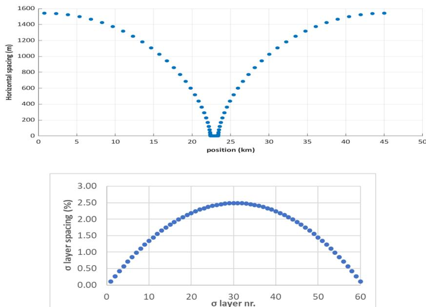
Figure 10: (a) Horizontal grid distribution for the model runs, using a fine grid in the centre where the sand waves are calculated and a coarser grid towards the lateral boundaries and (b) the vertical distribution of the  $\sigma$ -layers over the water column, showing the spacing of 60  $\sigma$ -layers down the water column. The spacing between the layers is small near the bed and surface, resulting in 8  $\sigma$ -layers at the lower 1 m and top 1 m.
