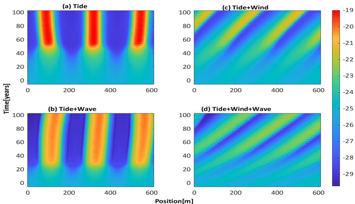
Figure 27: Sand wave profile development in the presence of tide (a), tide +wave (b), tide+ wind (c) and tide+ wind + wave (d) over 0.25 m symmetrical initial bed for 100 years. The vertical colour bar shows the bed level (m).
