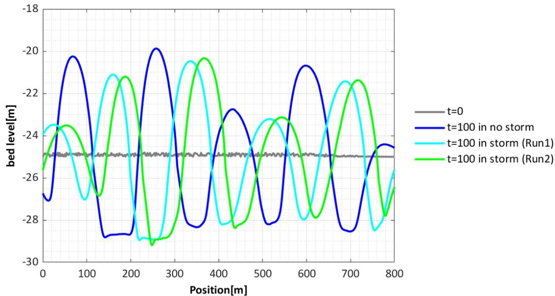
Figure 36: Sand wave profile in the no storm (blue) and two random intermittent storm conditions of 3 months/year (cyan and green) after 100 years at 25 m mean depth. The same randomly perturbed bed is used at t=0 (grey) for the simulations presented here.
