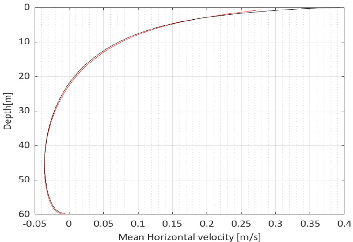
Figure 38: Mean Horizontal velocity at depth 60 for numerical settings- number of sigma layers (90 layers), horizontal distribution near the centre of the grid (1m) and hydrodynamic time step (0.1 minutes) (red) and - number of sigma layers (60 layers), horizontal distribution near the centre of the grid (2m) and hydrodynamic time step (0.2 minutes) (black)
