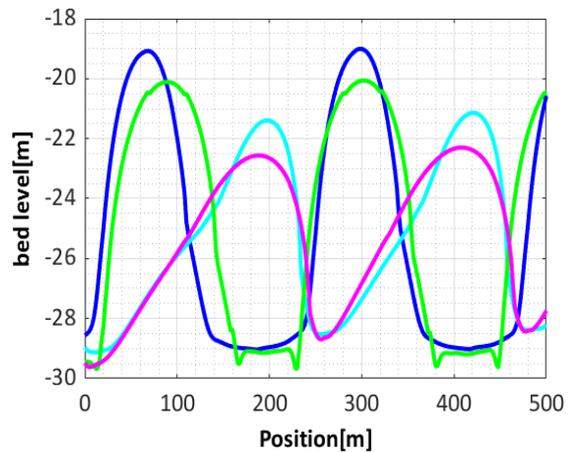
Figure 29: Sand wave profile in the presence of tide (blue), tide +wave (green), tide+ wind (cyan) and tide+ wind + wave (purple). The final sand wave profile is generated from 0.25 m initial amplitude sand wave (FGM=216 m) after the morphological development of 100 years.
