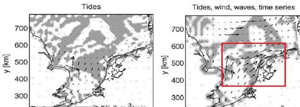
Figure 7: Eastward sand transport component and suspended load towards the Dutch coast using a model study ( Van Der Molen, 2002) and ten years of wind data at the Texelhors meteorological station, due to (A) Tides, (B) Tides, wind and waves.
