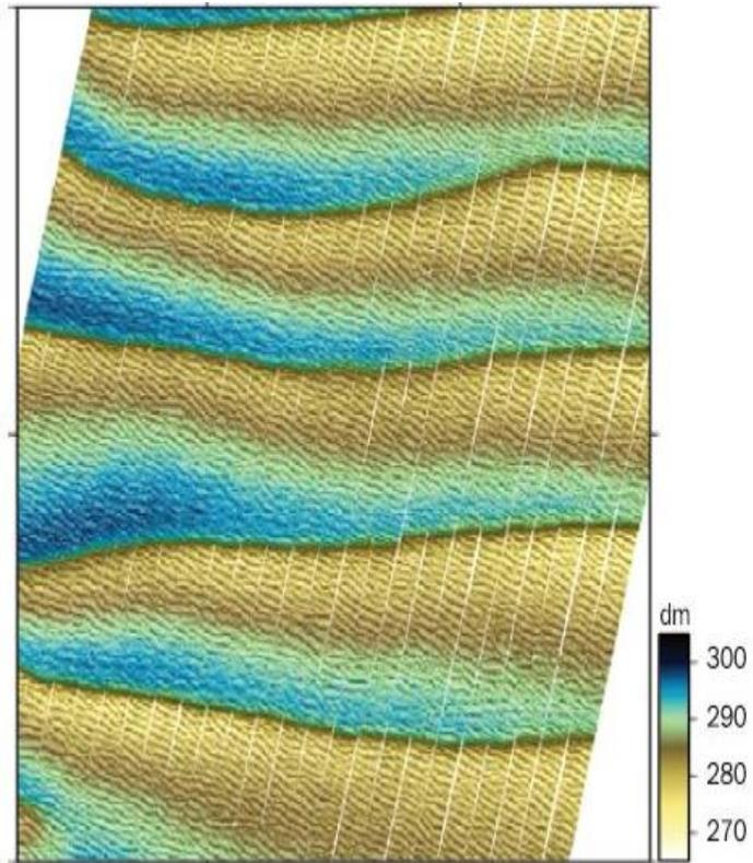
Figure 4: Interpolated survey images of 1 km<sup>2</sup> area, showing sand waves and megaripples near Egmond, Netherlands. Depths are given in decimeters to MSL. (Van Dijk et al., 2008)
