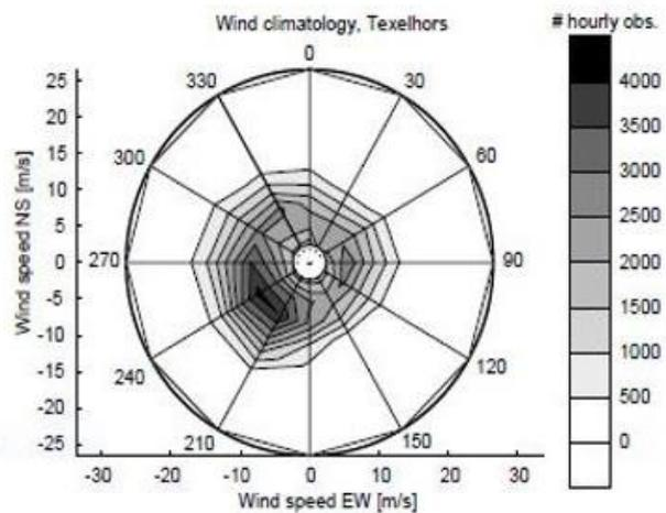
Figure 12: Wind climate derived from the 10-year time series of wind observations from Texelhors (KNMI, Verkaik, pers.comm.). Contours denote the observed number of hourly occurrences. Winds are from the direction (in compass degrees from north) indicated in the figure.
