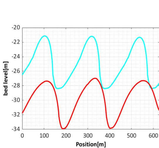
Figure 31: The sand wave field at 25m (cyan) and 30m (red) water depth in tide and severe wind after t=100 years.
