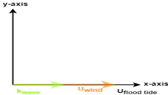
Figure 8: Definition sketch (top view) of the direction of tidal current (black), wind (orange) and wave vector (green).
