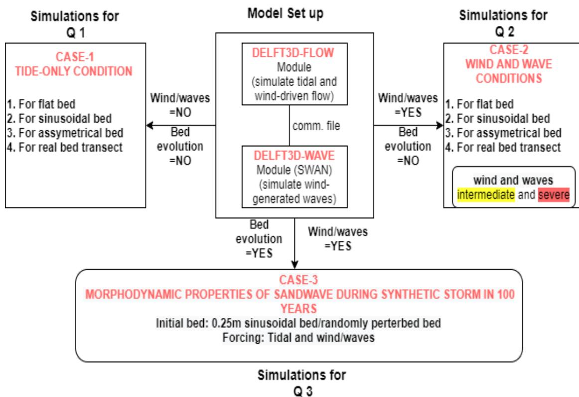
Figure 3: A schematic diagram for the approach used.
