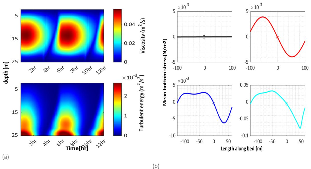
Figure 15: (a) Variation of vertical eddy viscosity (top) and turbulent energy (bottom) at crest position with tide duration. (b)Variation of tidally averaged bottom stress with sand wave evolution: a flat bed (black), 0.25m symmetrical sand wave (red), 0.25m asymmetrical sand wave (blue), real bed (cyan). The circle shows the stress at the crest position of sand waves (x=0m). It is in the presence of tide-only conditions.
