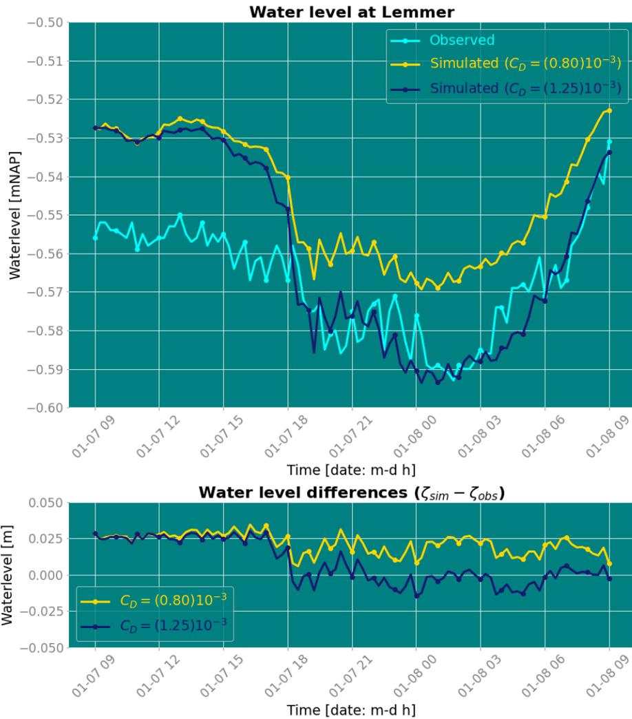
**Figure B.34:** Water levels at Lemmer during event 6 Bft S (B) at a local optimal  $C_D$  of  $0.80 \times 10^{-3}[-]$  (KGE= 0.83) in comparison to the uniform optimal  $C_D$  of  $1.25 \times 10^{-3}[-]$  (KGE= 0.54)
