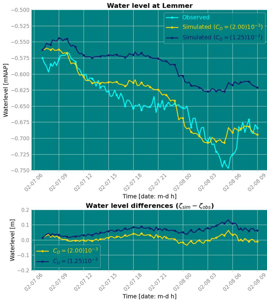
**Figure B.33:** Water levels at Lemmer during event 6 Bft S (B) at a local optimal  $C_D$  of  $2.00 \times 10^{-3}$  [–] (KGE= 0.91) in comparison to the uniform optimal  $C_D$  of  $1.25 \times 10^{-3}$  [–] (KGE= 0.26)
