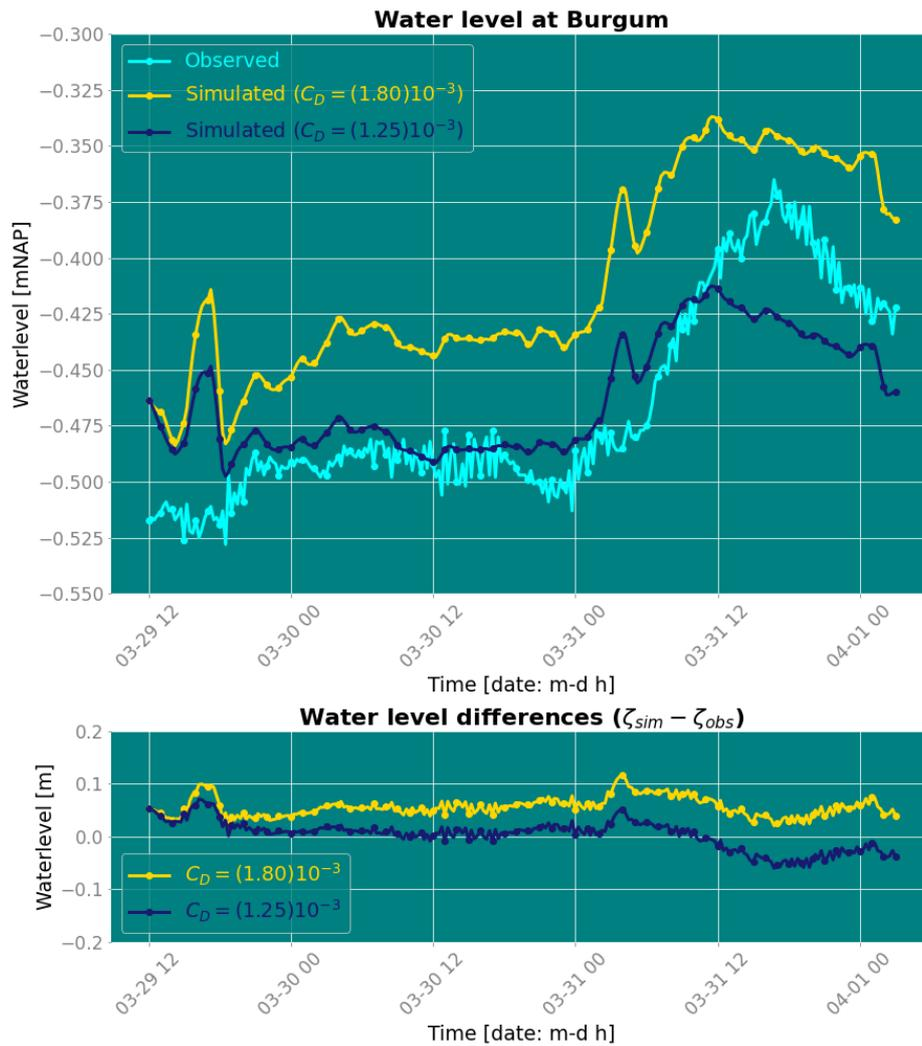
**Figure B.44:** Water levels at Burgum during event 6 Bft S (B) at a local optimal  $C_D$  of  $1.80 \times 10^{-3}[-]$  (KGE= 0.84) in comparison to the uniform optimal  $C_D$  of  $1.25 \times 10^{-3}[-]$  (KGE= 0.24)
