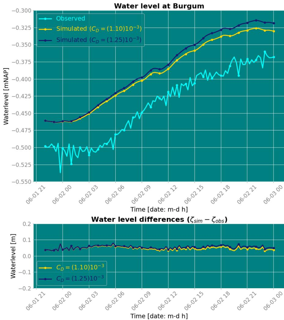
**Figure B.43:** Water levels at Burgum during event 6 Bft S (B) at a local optimal  $C_D$  of  $1.10 \times 10^{-3}$  [–] (KGE= 0.87) in comparison to the uniform optimal  $C_D$  of  $1.25 \times 10^{-3}$  [–] (KGE= 0.84)
