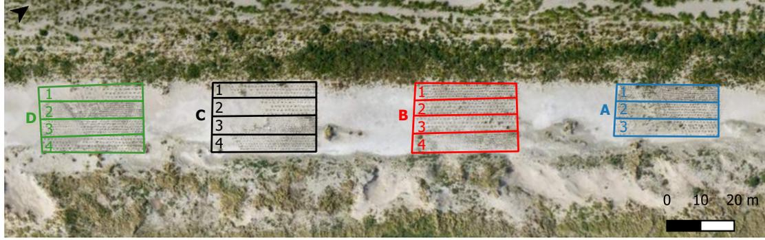
Figure 3.5: Aerial photo (Gulden, 2018) of most northern part of valley, showing the set-up of the reed bundle experiment. Fields are indicated as A, B, C and D, strips are indicated with numbers 1, 2, 3 and 4. Aerial photo taken in Sep 2018
