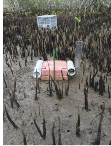
(a) Close up of one pressure gauge attached to the anchors (b) Placement of the pressure gauges and conductivity sensor in the field
