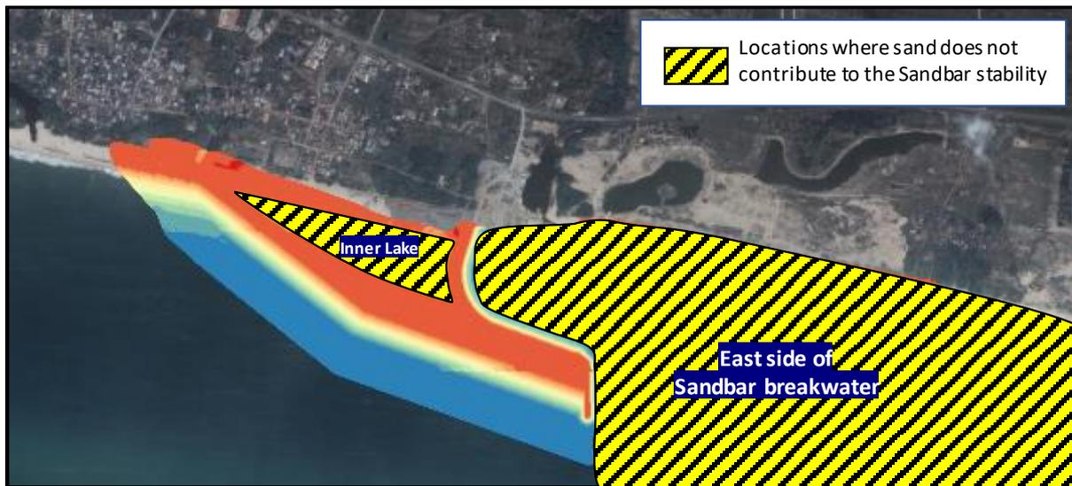
Figure 2.8: Locations in the area of interest where sediment nourished inside the design profile but is moved/transported outside the design profile by natural processes is considered as a sediment loss: the Inner Lake and at the East side of Sandbar Breakwater which is indicated by the black-yellow polygons.
