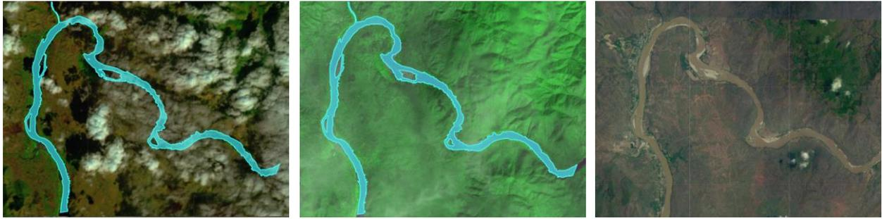
**Figure 4.15** – Typical resulting river polygon for the Thanlyin River nearby Khe Hpyu, Myanmar, based on Landsat 8 and Sentinel-2 data respectively. The third image (right) is a standard google maps image (source: Map data © 2018 Google).
