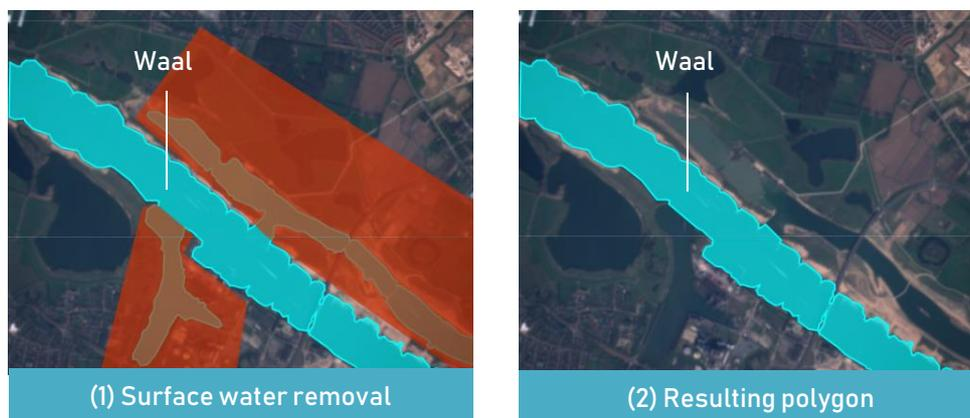
**Figure 3.14** – Demonstration of the exclusion of surface water for a segment of the Waal.
