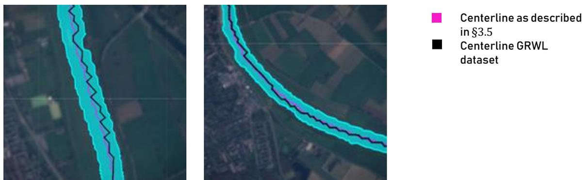
**Figure 4.5** – Comparison between the quality of the centerline of the approach as seen in §3.5 (purple) and the GRWL dataset (black).
