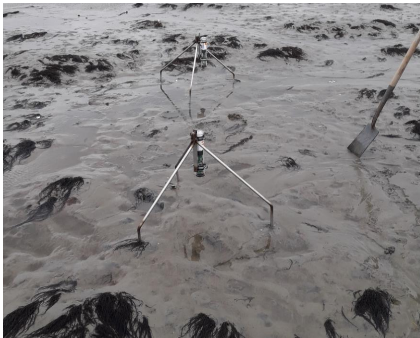
Figure 4.2: New frame of the ASED-sensor with three poles in the bed.
