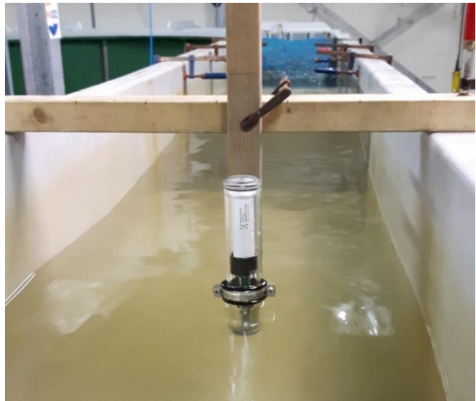
Figure 2.8: Set-up of the ASED-sensor for the waves and current measurements
