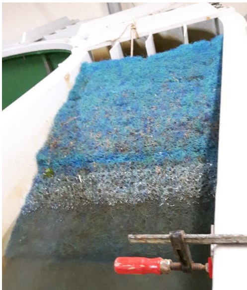
Figure 2.7: Wave break material for damping the waves
