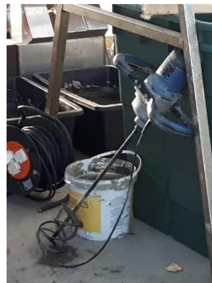
Figure 2.14: Mixer powered by an electrical drilling machine
