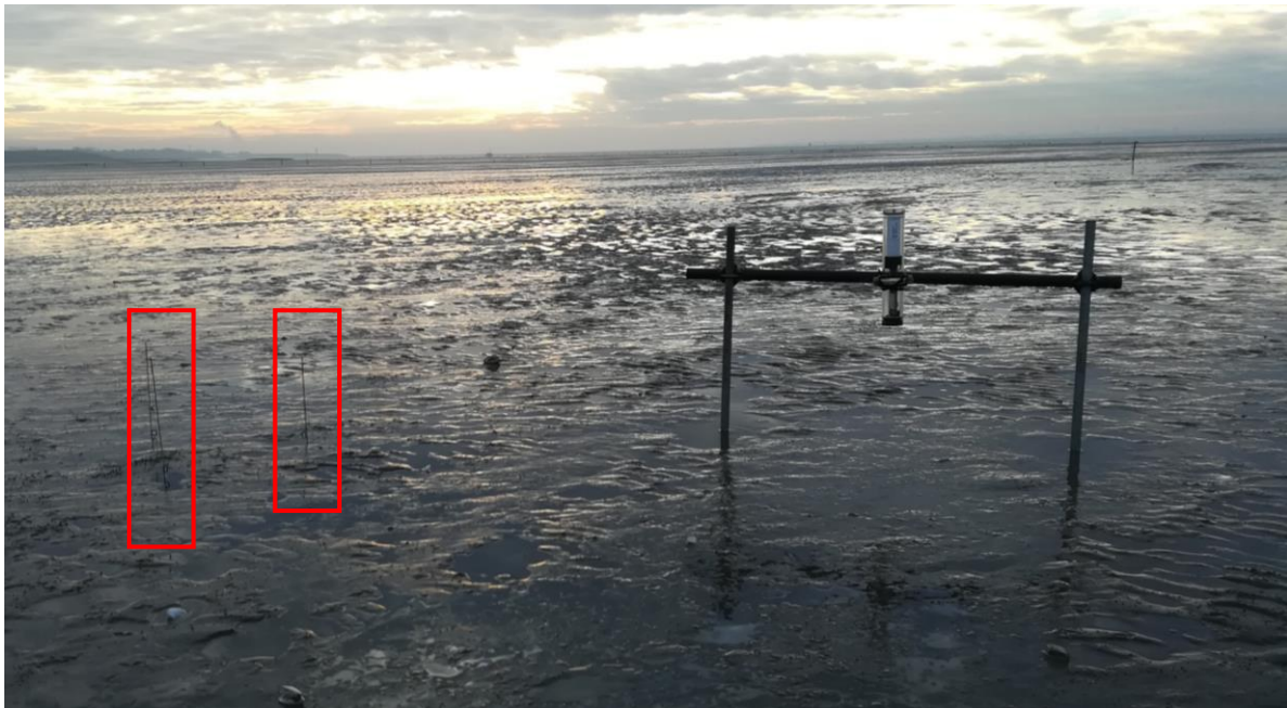
Figure 2.15: Three erosion pins (two erosion pins in the left red box) in the Western Scheldt experiment
