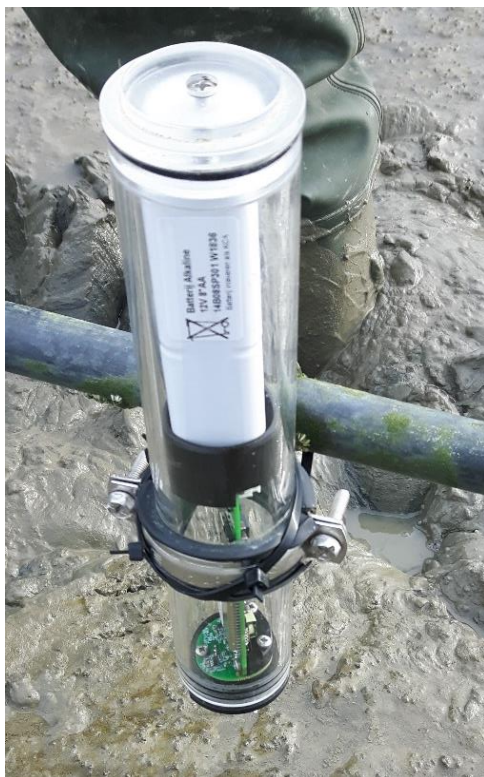
Figure 2.1: The waterproof transparent polyester case of the ASED-sensor
