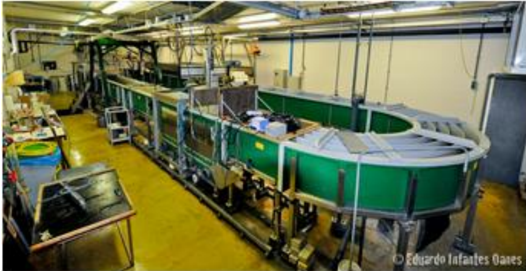
Figure 2.6: The wave flume of NIOZ (NIOZ website)
