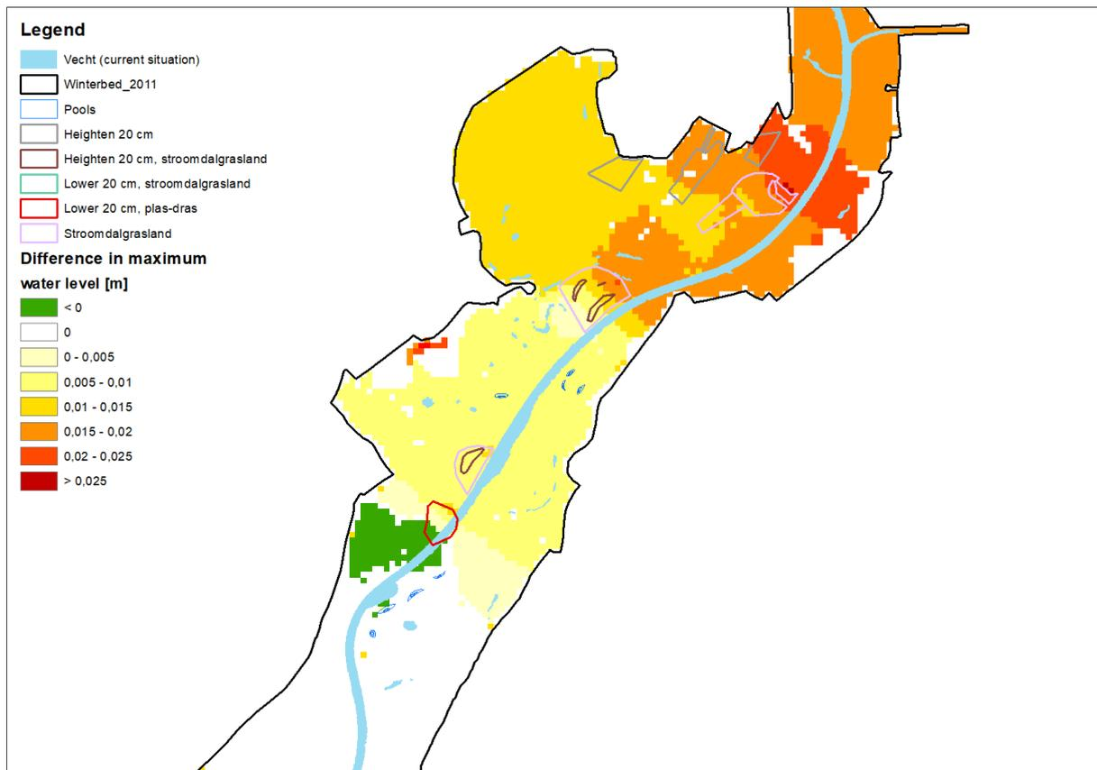
Figure 64. Difference in maximum water level [m] at Rheezermaten (only measures at Rheezermaten implemented). A positive value indicates a higher maximum water level, while a negative value indicates a lower maximum water depth.
