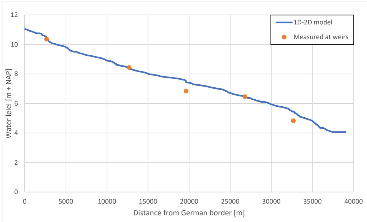
Figure 14. The maximum water levels of the River Vecht in longitudinal direction after the winter bed calibration ( $T=10$ ).
