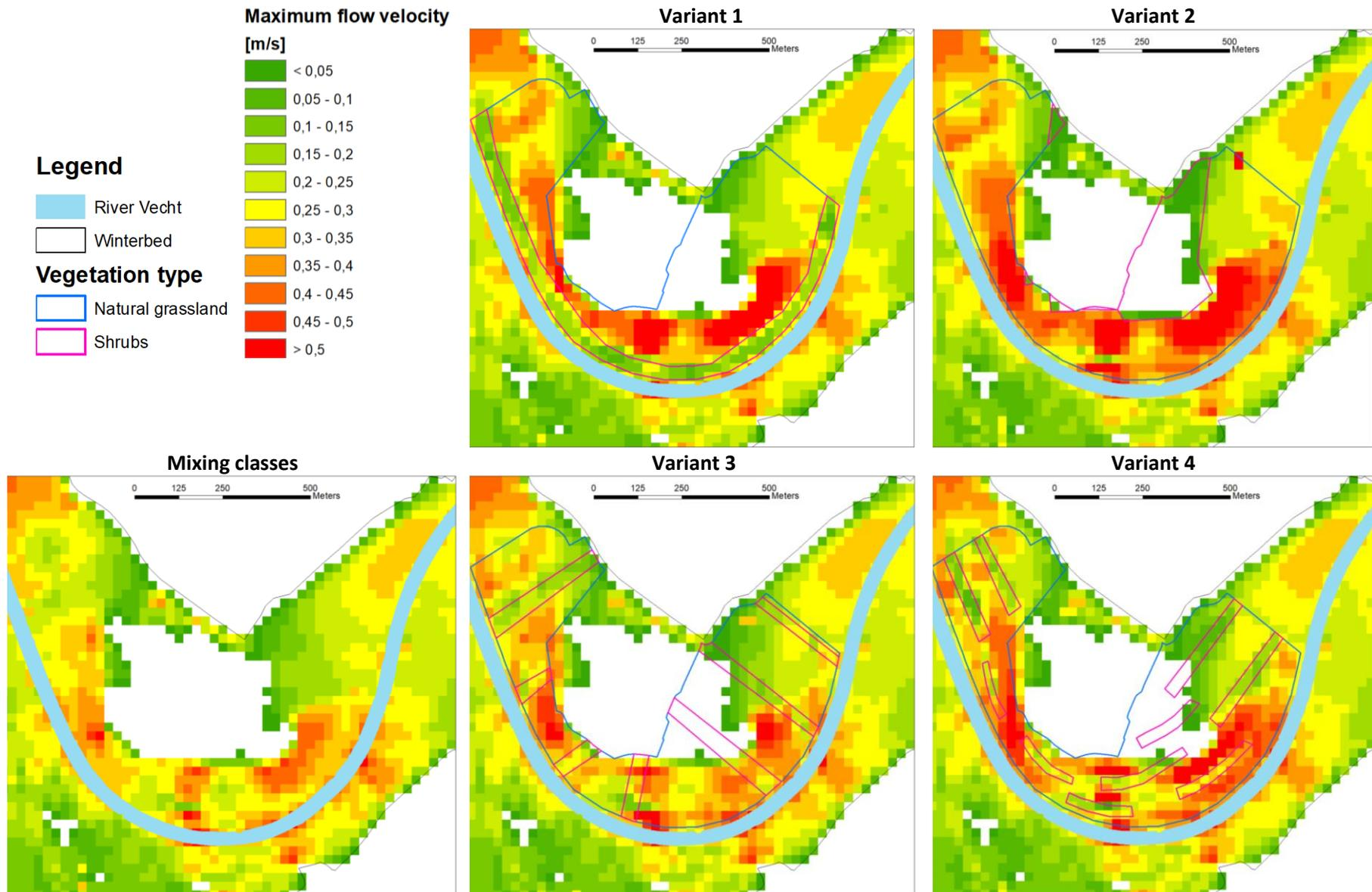
Figure 54. Maximum flow velocities [m/s] on the lot with mixing class 80/20 for the different scenarios.
