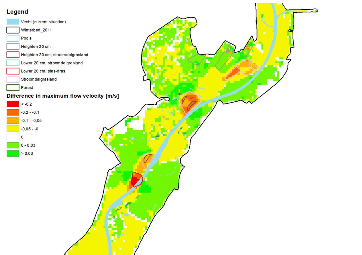
Figure 68. The differences in maximum flow velocity at Rheezermaten (both projects implemented). A negative value indicates a lower flow velocity after the implementation of the measures, a positive value indicates a higher flow velocity.
