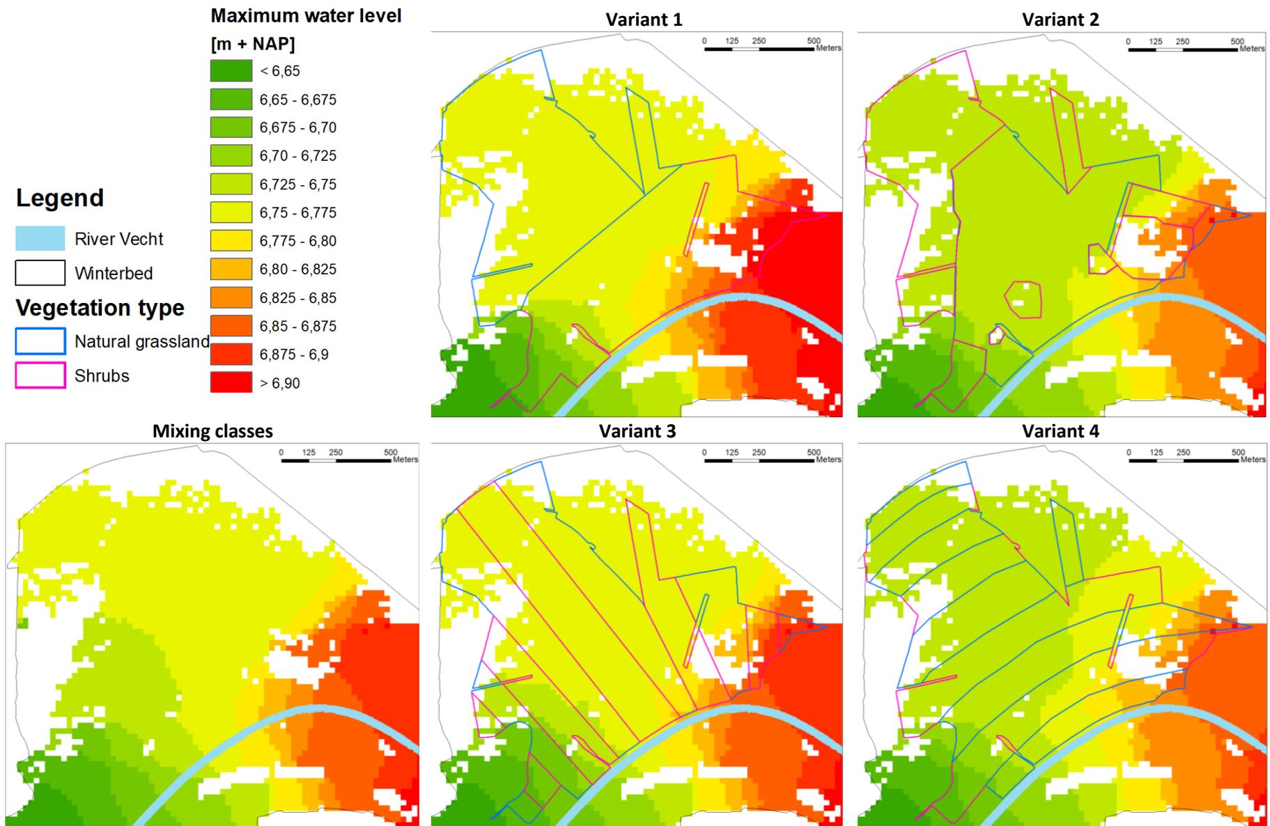
Figure 56. Maximum water levels [m + NAP] on the lot with mixing class 50/50 for the different scenarios.
