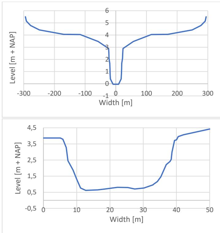
Figure 6. Cross-sections in the 1D hydraulic SOBEK model: a symmetric main channel cross-section (upper) and a asymmetric side channel (lower).
