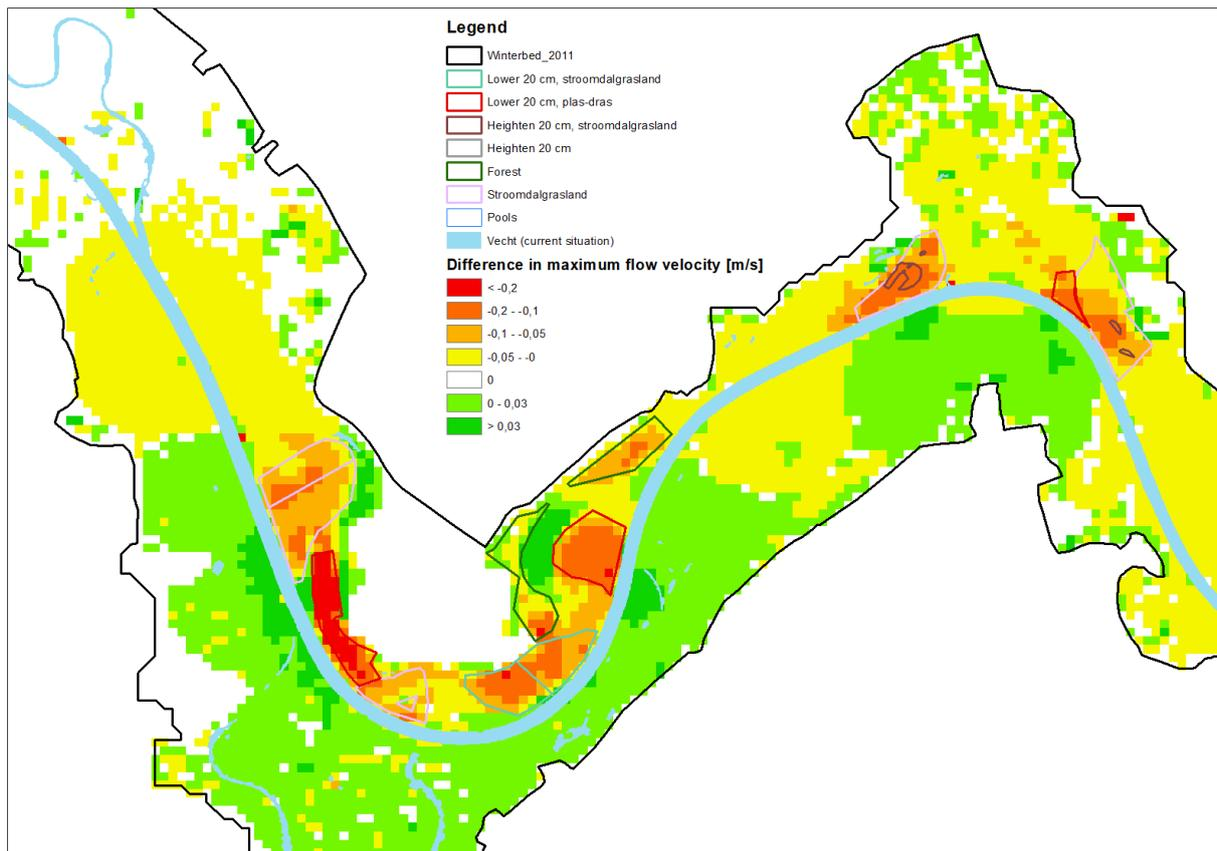
Figure 66. The differences in maximum flow velocity at Karshoek-Stegeren. A negative value indicates a lower flow velocity after the implementation of the measures, a positive value indicates a higher flow velocity.
