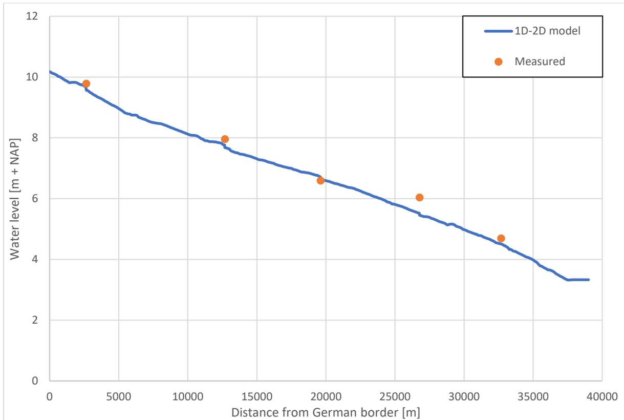
Figure 15. The maximum water levels of the River Vecht in longitudinal direction after the validation ( $T=1$ ).
