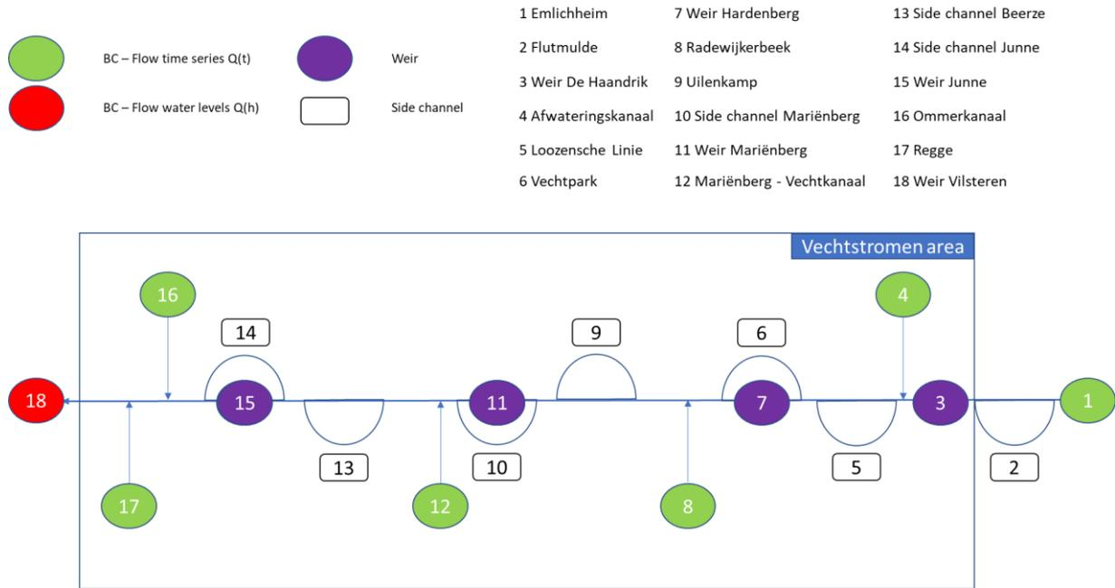
Figure 5. Schematisation of the network in SOBEK 2. Only the five (out of eighteen) largest lateral flows are shown.
