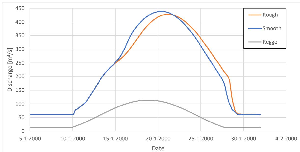
Figure 24. Discharge [m³/s] at the downstream border of the area of R.W.A. Vechtstromen for the rough and smooth scenario.
