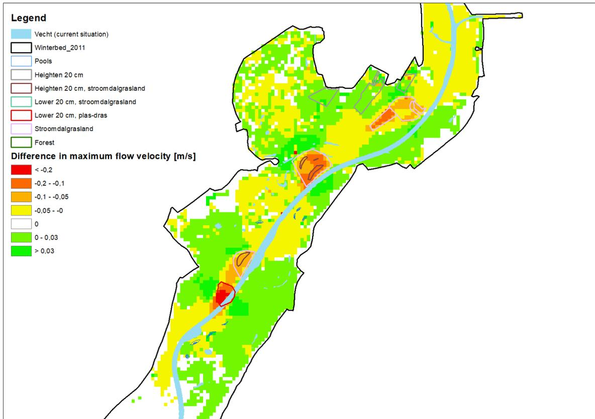
Figure 67. The differences in maximum flow velocity at Rheezermaten (measures at Rheezermaten only). A negative value indicates a lower flow velocity after the implementation of the measures, a positive value indicates a higher flow velocity.
