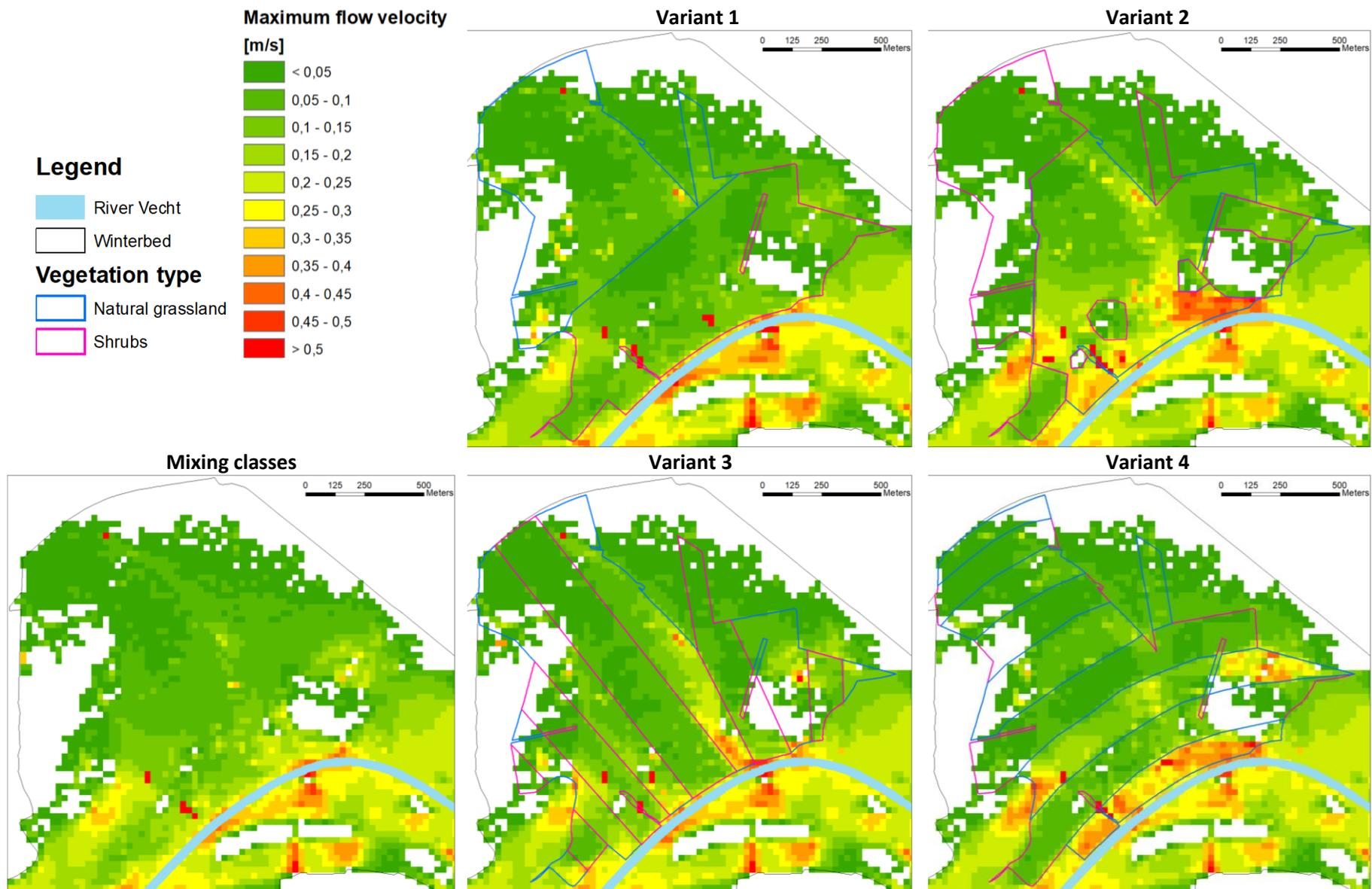
Figure 58. Maximum flow velocities [m/s] on the lot with mixing class 50/50 for the different scenarios.
