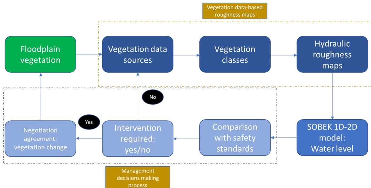
Figure 2. Workflow that shows the different steps to determine if an intervention in the vegetation in the floodplains is needed regarding the safety standards.
