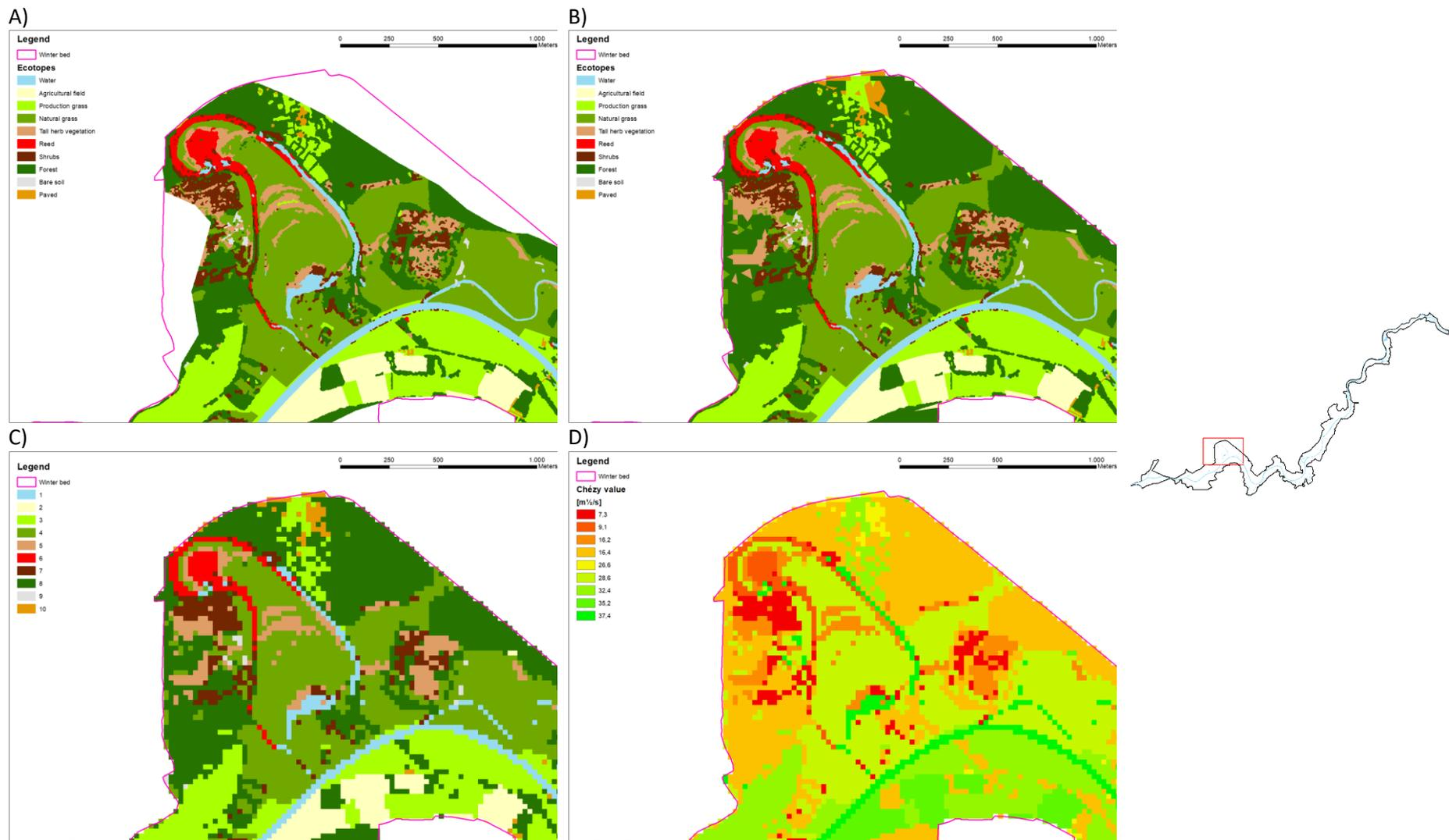
Figure 12. The process of generating a roughness grid for the hydraulic 1D-2D model. First, the ecotopes map (A) is completed with data from the LGN map, resulting in an ecotopes map with data for every location in the winter bed (B). The ecotopes map is then converted into a raster (25×25 m) with codes corresponding to the vegetation classes (C), which is then converted into a grid with Chézy values (D).
