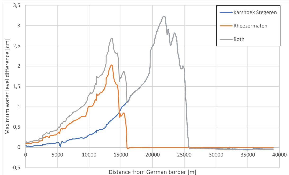
Figure 62. The difference in water level as result of the implementation of the measures of the planned measures compared to the current situation.
