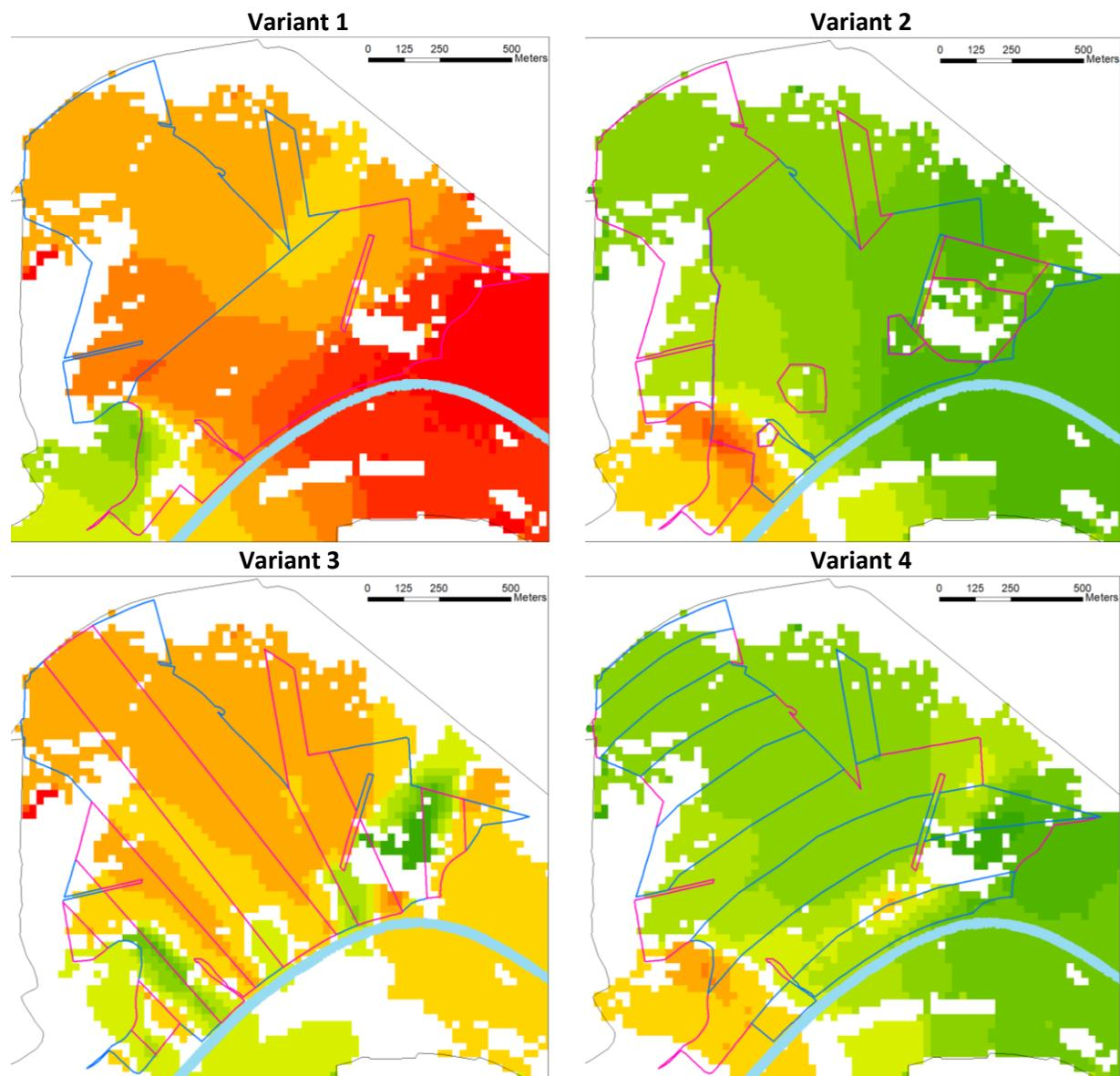
Figure 57. Difference in maximum water levels [m] for the different scenarios on the lot with mixing class 50/50 compared to the model run with the mixing classes.
