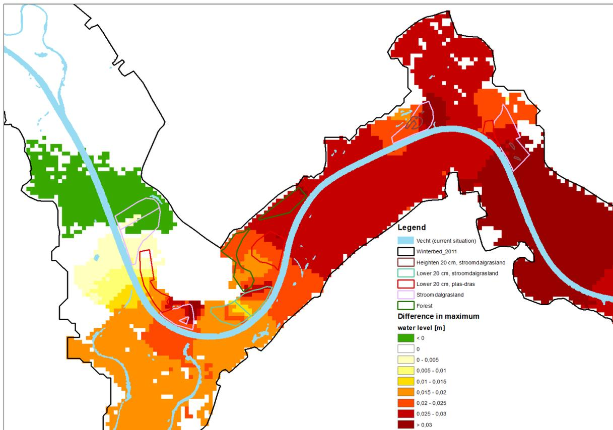
Figure 63. Difference in maximum water level [m] at Karshoek-Stegeren. A positive value indicates a higher maximum water level when the measures at Karshoek-Stegeren are implemented, while a negative value indicates a lower maximum water depth.
