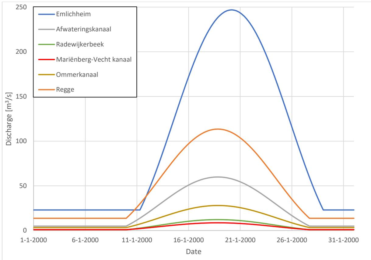
Figure 8. The upstream boundary condition ( $Q-t$  relation) and five largest lateral flows ( $T=200$ ).
