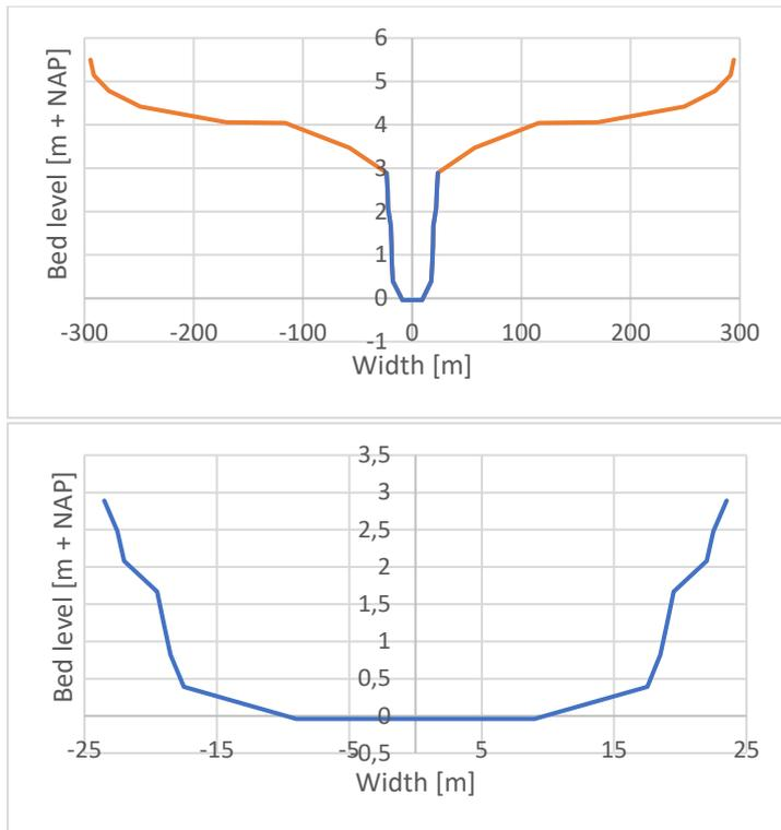
Figure 9. A cross-section in the 1D-2D part of the hydraulic SOBEK model: the original main channel cross-section (upper) where distinction is made between the main channel (blue) and winter bed (orange) and the same cross-section after removing the winter bed (down).
