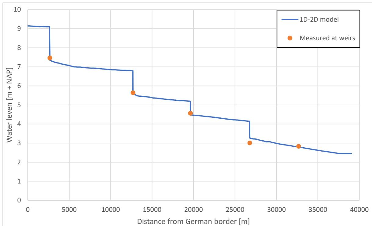
Figure 13. The maximum water levels of the River Vecht in longitudinal direction after the main channel calibration ( $T=1/4Q$ ).
