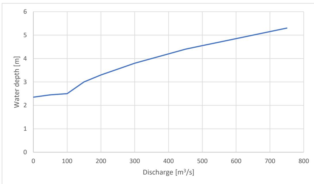
Figure 7. Downstream boundary condition (Q-h relation).
