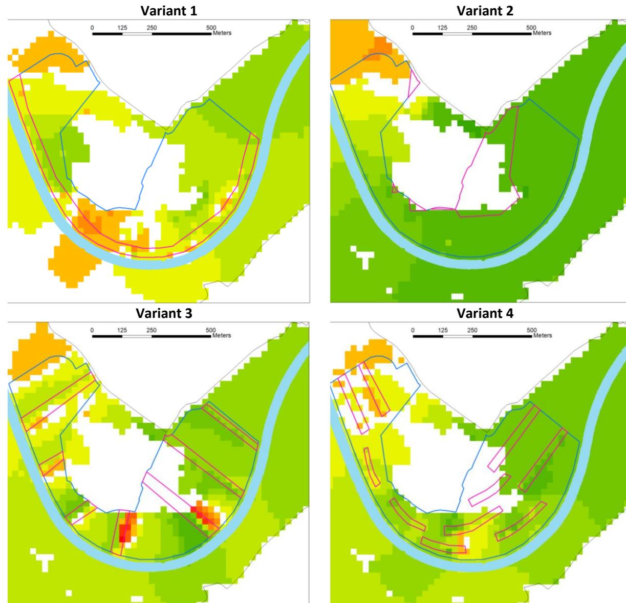
Figure 53. Difference in maximum water levels [m] for the different scenarios on the lot with mixing class 80/20 compared to the model run with the mixing classes.
