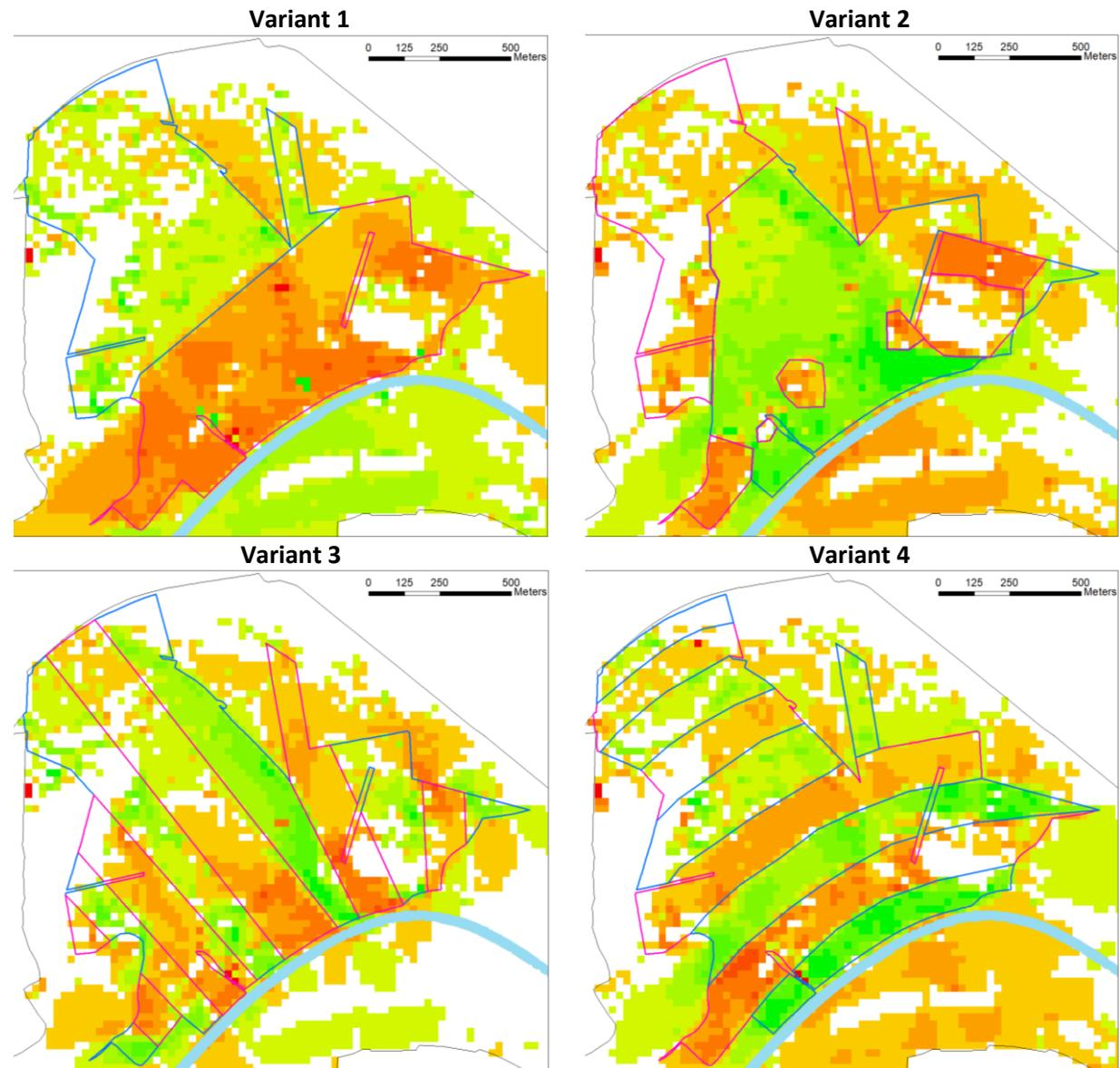
Figure 59. Difference in maximum flow velocity [m/s] for the different scenarios on the lot with mixing class 50/50 compared to the model run with the mixing classes.
