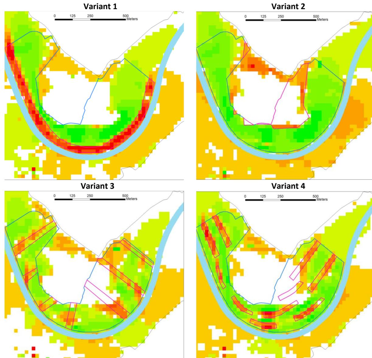
Figure 55. Difference in maximum flow velocity [m/s] for the different scenarios on the lot with mixing class 80/20 compared to the model run with the mixing classes.
