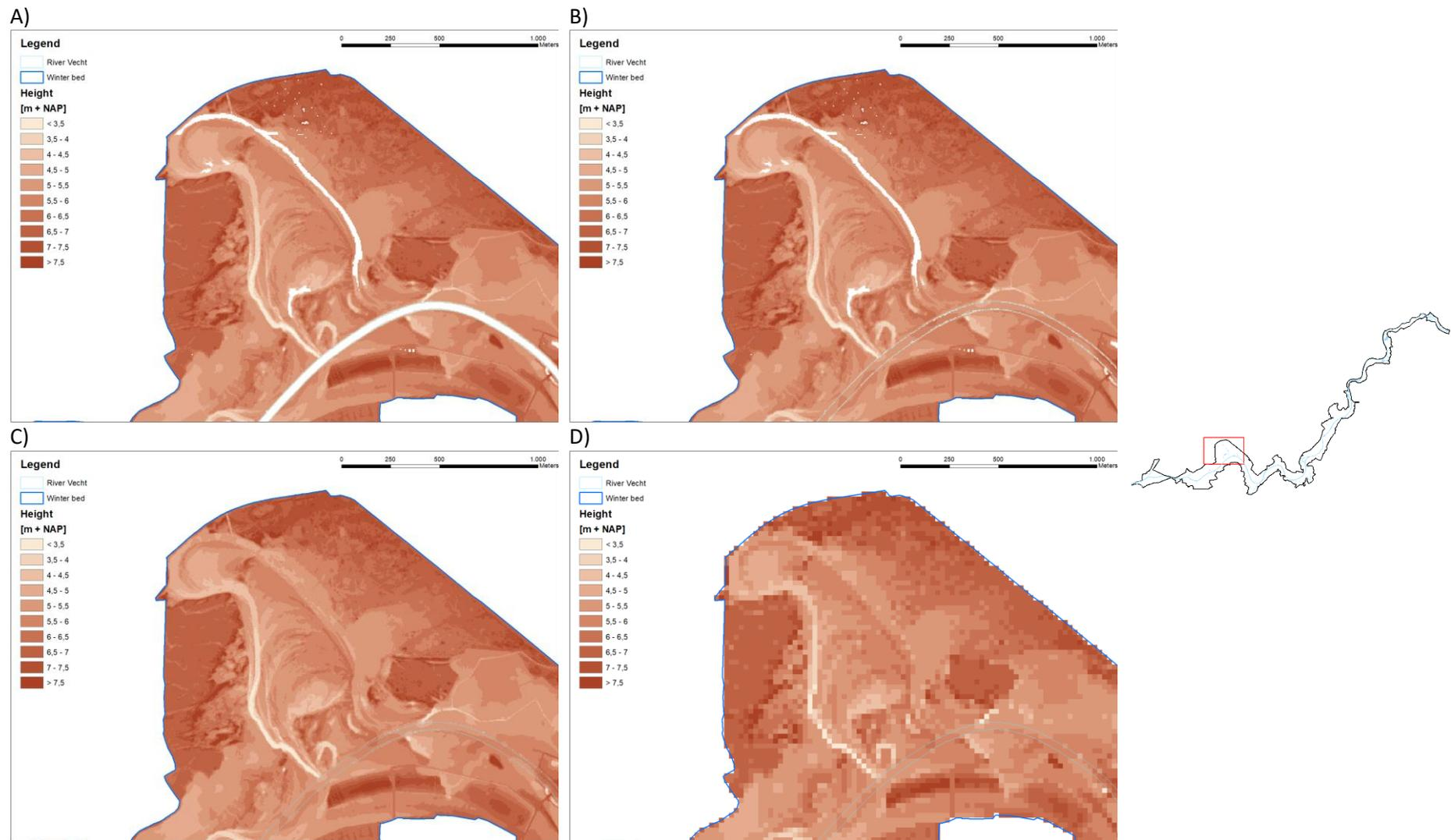
Figure 11. The process of generating an elevation grid for the hydraulic 1D-2D model. First, the missing values of the main channel in the AHN map (A) are replaced by the values of the height of the summer dikes surrounding the main channel (B). After this, the remaining no-data values are interpolated (C). Finally, the 5x5 m height map is converted in a 25x25 m grid (D).
