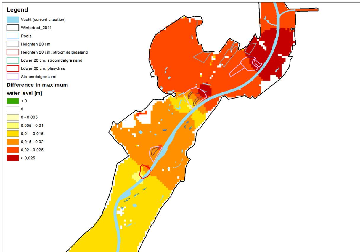
Figure 65. Difference in maximum water level [m] at Rheezermaten (both the measures at Rheezermaten and Karshoek-Stegeren implemented). A positive value indicates a higher maximum water level, while a negative value indicates a lower maximum water depth.
