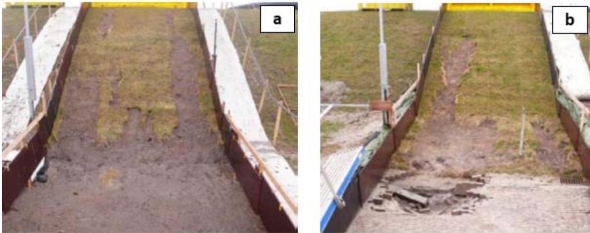
Figure 2.6 Grass cover erosion at the slope and the landward toe at test sections (a) Afsluitdijk 1 and (b) Afsluitdijk 2 after wave overtopping tests with maximum mean overtopping discharges  $q_m = 75$  l/s/m and  $q_m = 10$  l/s/m. Figures obtained from Van der Meer (2014).
