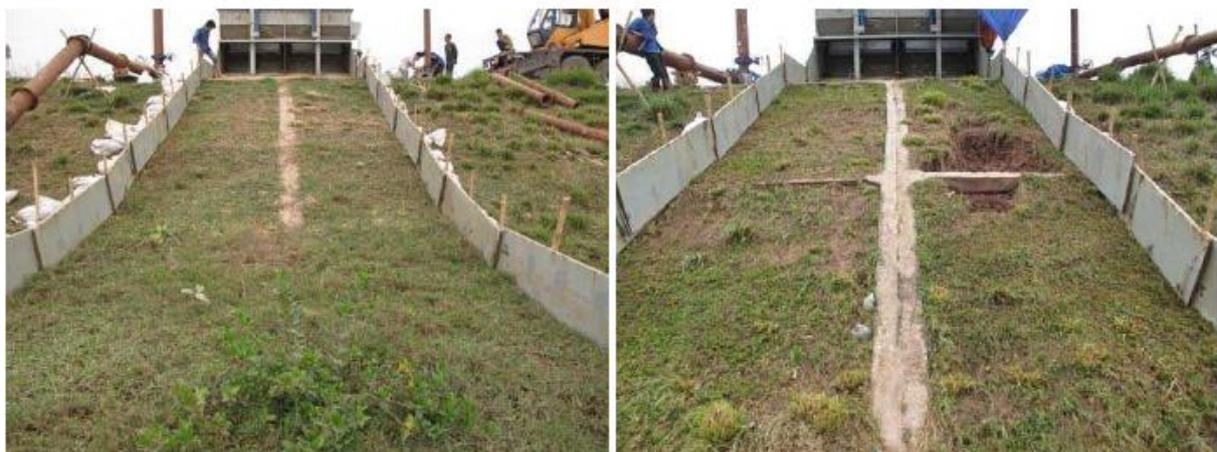
**Figure A1.1** Presence of a concrete frame with horizontal and vertical beams in the grass revetment at Thai Tho, Vietnam, before testing (left) and after testing (right). Figure adapted from Le (2011).
