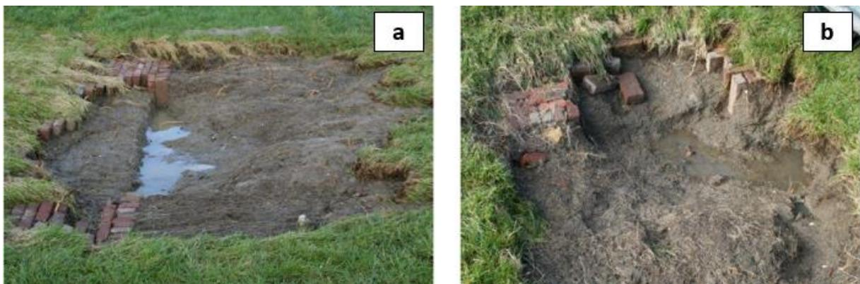
Figure 2.5 Grass cover erosion at the landward toe at test sections (a) Boonweg 1 and (b) Boonweg 2 after wave overtopping tests with a maximum mean overtopping discharge  $q_m = 75$  l/s/m. Figures obtained from Van der Meer (2014).
