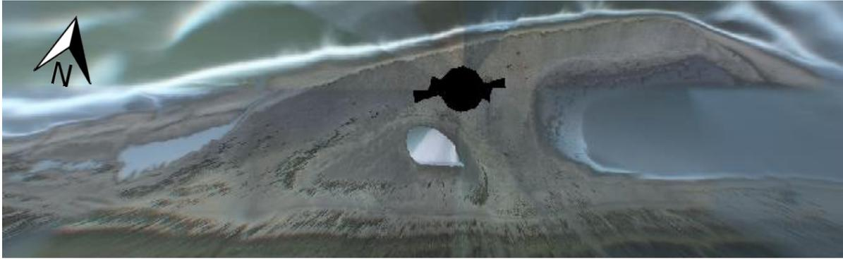
Figure 17, 12-images-merged-rectified picture of the Sand Motor 27-10-2018. The pictures are made from the Argus station at the centre of the Sand Motor. The black area on this picture is outside the range of the cameras. The green dots on the picture is vegetation growing on the Sand Motor.
