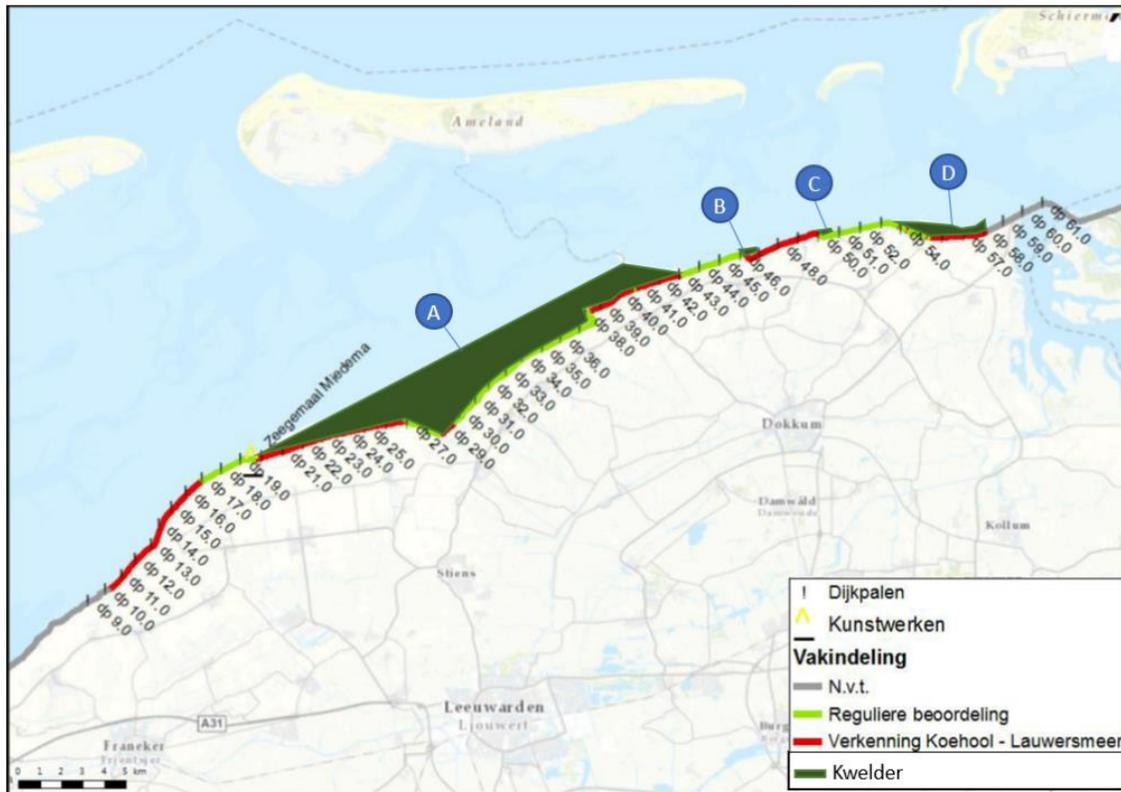
Figure 4 - Salt marshes (in dark green) along the Wadden Sea dike between Koehool and Lauwersmeer. Dike poles are used as location marker (Alterra, 2012b; Witteveen+Bos, 2017a)
