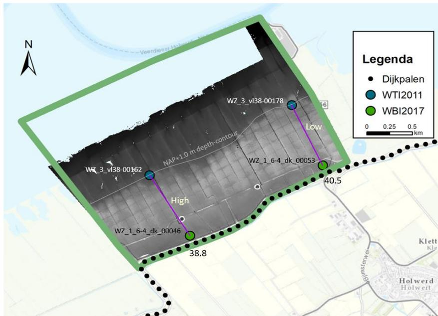
Figure 20 - The transects that were modeled from a WTI2011 location to a WBI2017 location (Rijkswaterstaat WVL, 2018b). The left one had high wave reducing potential and the right one low wave reducing potential. The elevation map represents the geometry of Holwerd West in 2005, in which the WTI2011 locations are approximately located at the NAP+1.0 m depth contour, at GHW level (Figure created from Klein and Kroon, 2011).
