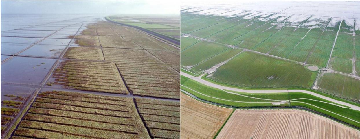
Figure 2 - Semi-artificial salt marshes have developed in front of the Wadden Sea dike, supported by salt marsh works (Aerial pictures by Jaap de Vlas) (van Duin et al., 2013); (Steezel et al., 2019).
