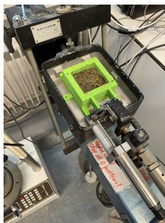
Figure 1: Direct shear test apparatus with vegetated sample
