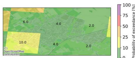
Figure 1: Output of the W2O model for Udenhout (Municipality of Tilburg). Probability of exceedance is defined as percentage of ensemble members that predict an inundation depth of more than 10 mm.
