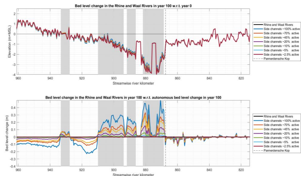
Figure 1: Bed level change after 100 years w.r.t. year 0 (top) and w.r.t. autonomous bed level change (bottom).
