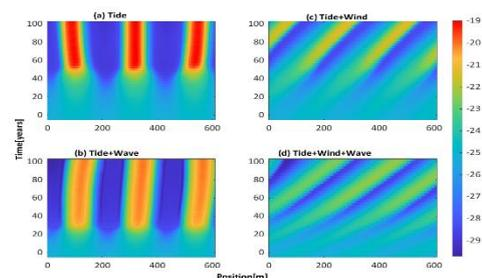
Figure 1: Sand wave profile development in the presence of tide (a), tide + wave (b), tide + wind (c) and tide + wind + wave (d) over 0.25 m symmetrical initial bed for 100 years. The vertical colour bar shows the bed level (m).
