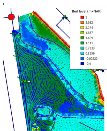
Figure 1: Example of 2D flow through a retention area.
